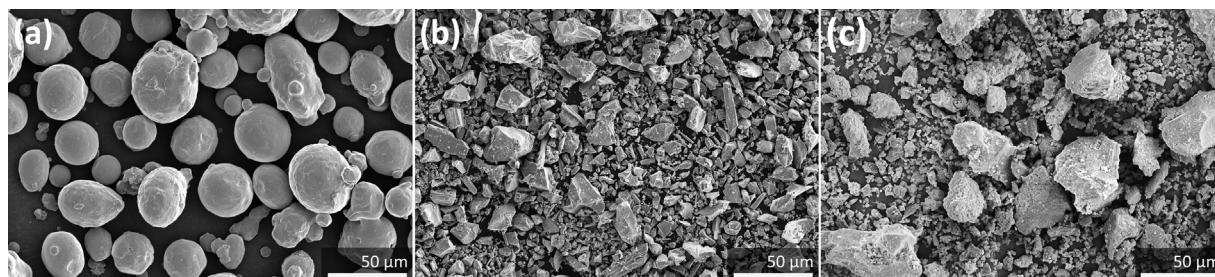
Fig. 1. The morphologies of (a) iron, (b) manganese, and (c) akermanite powders.
