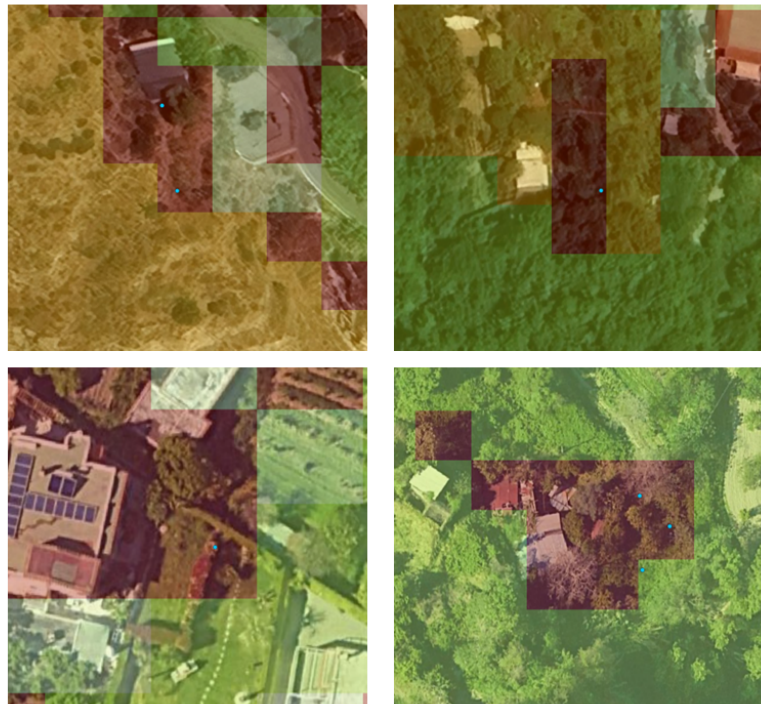
Figure 5.3: Example of possible InSAR scatterers overlapping pixels classified as urbanised land cover (red), although they may actually belong to other local land cover classes.
