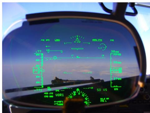
Figure 9.3: Head-Up-Display interface<sup>8</sup>
