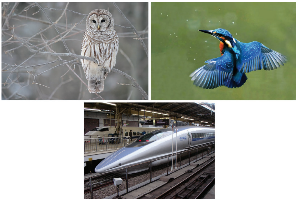
Figure 23.8 Shinkansen 500 series train, kingfisher's beak, and closeup of owl feathers to show the sound-damping leading edge
