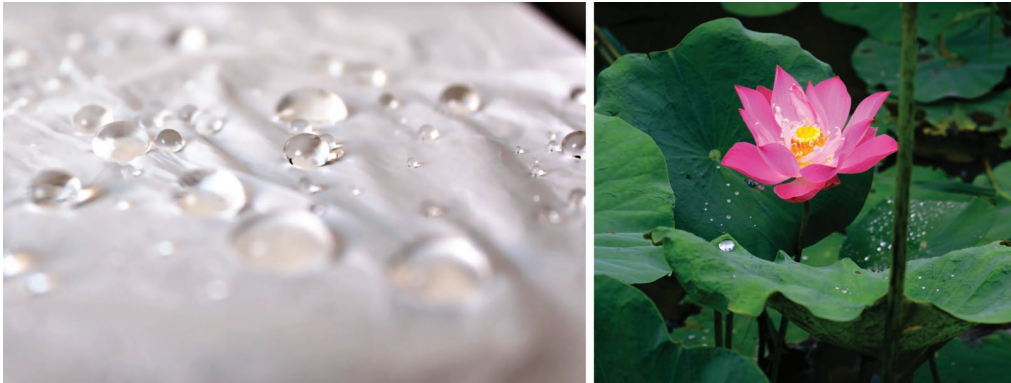
Figure 23.1 Amphitex waterproof and recyclable mono-material fabric (left) and the lotus leaves that inspired them (right)
