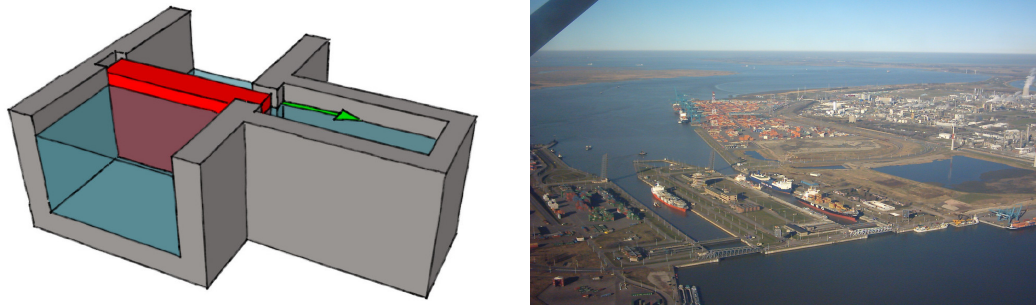
Figure 19: Left: Illustration of a Horizontal Translation Gate, Right: Berendrecht locks, [BEL]
