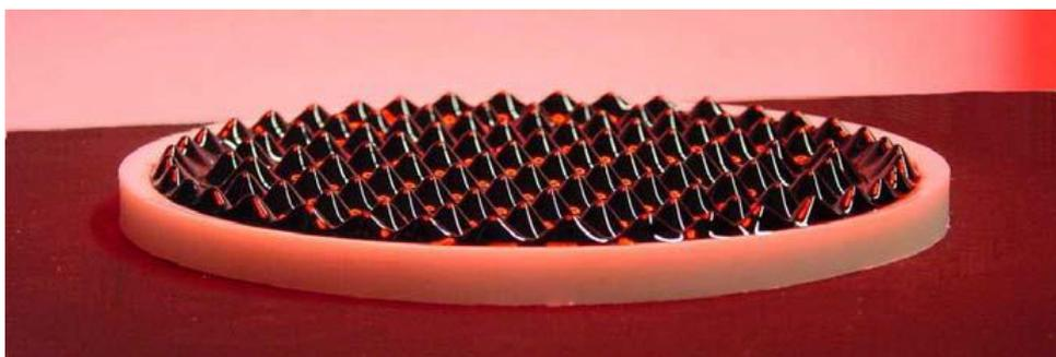
Fig. 2-26. The picture presents the Rosensweig instability in a Teflon vessel with a diameter of 12cm . The magnetic field shows to be above the critical value  $H > H_c$  since surface instability is observed.
