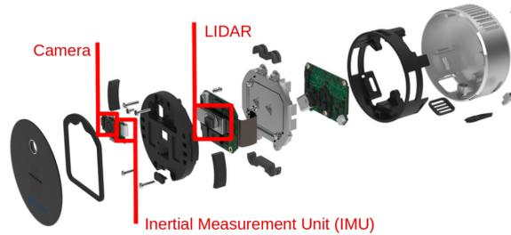
**Figure 1-3:** Expanded view of all the components of the Intel L515 Sensor. The sensors contains a camera, Lidar and Inertial measurement unit [10].
