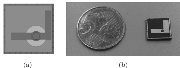
Figure D.1: Dual-band single L-bar patch antenna. (a)- simulated vertically-polarised (VP) variant and (b)- fabricated prototype.
