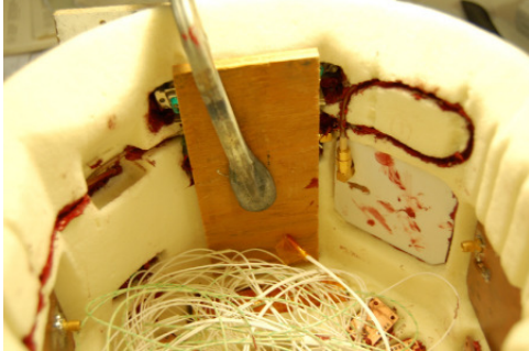
Figure 15: First, the beacon package is mounted, using red silicone as glue. It is located entirely outside the metal cage of the capsule electronics and close to its antennas. This insures maximum survival probability in case of a capsule crash.
