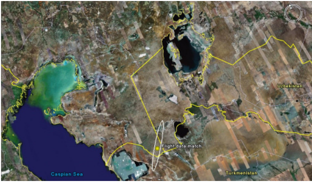
Figure 26: Estimated landing area of Fotino. Several bodies of water are proximate, so a wet landing may have occurred. The ground station was located too far upstream (over the horizon) to receive any telemetry.
