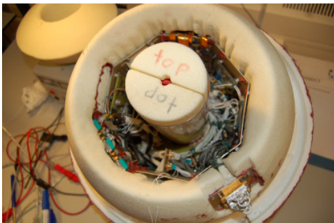
Figure 23: The parachute is transferred into the capsule's PET cylinder
