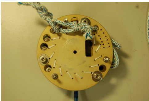
Figure 13: Different views of the charged flight parachute ejection system with pyro. The springs are held in place by three temporary bolts around the plates' circumference. The springs force causes elastic deformation visible to the naked eye, highlighting the minimalistic use of material.
