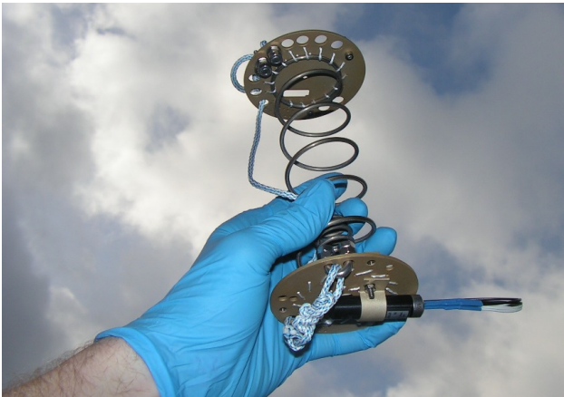
Figure 11: The parachute ejection system with unloaded springs. The central short spring is to break the capsule heatshield, the long spring then accelerates the chute away from the capsule
