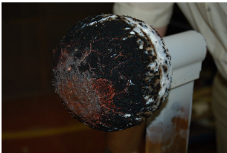
Figure 27: Fotino heatshield model after re-entry test in Plasmatron 20 appears charred and could have possibly blocked the ARGOS transmission signal. Conductivity measurements made on the charring seem to indicate likelihood of such a blockage is small.
