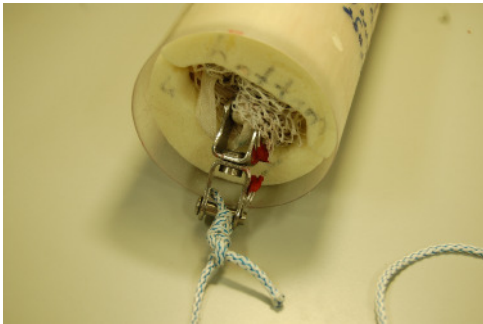
Figure 22: The parachute is folded and placed inside a foam sabot and stored in a PET cylinder. The bridle is connected to it by a swivel system to decouple parachute and capsule spinning.
