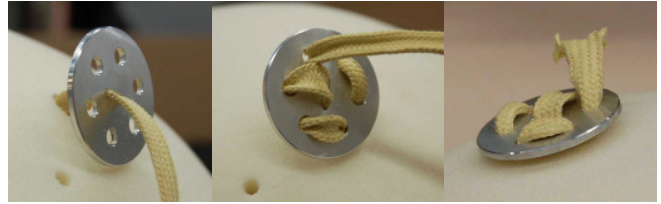
Figure 18: Close-ups of the fixation process of one of the anchor plates. Anchoring across the compressible PU core will also help to reduce the shock of the parachute opening.
