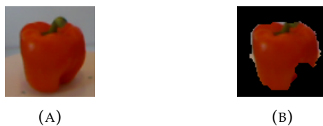
FIGURE 4.16: The masks as used in the Pick-and-Place dataset are noisy to some extent. Here, an extreme example is depicted. In experiment 3.1, an effort is made to investigate the effects of this noise on the performance. In all other experiments, the masked images are being used.
