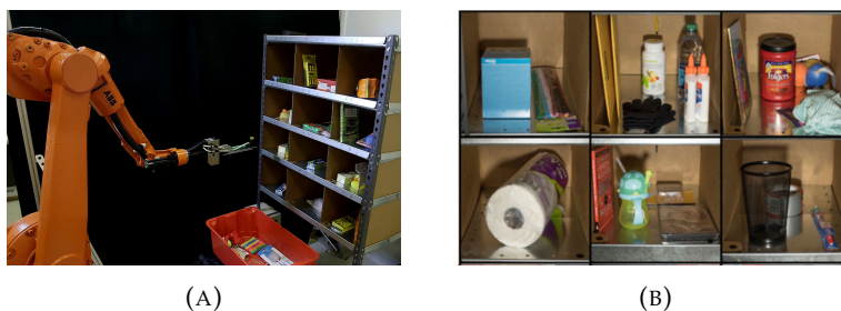
FIGURE 1.1: (A) Example of a pick-and-place scenario in a warehouse setting. Adapted from [51]. (B) Example of shelves from which a specific object has to be picked up. Adapted from [13] and edited.
