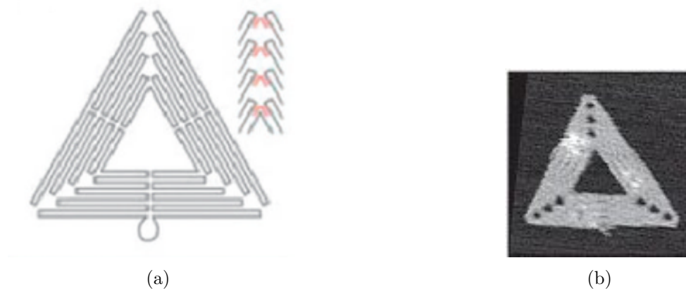
Figure A.1: a) Schematic and b) AFM representation of Rutherford triangles. In Figure a) the linkers are shown with red colour and most of the structure is composed of dsDNA, including a hairpin at the bottom side of the triangle. Adapted from [82].
