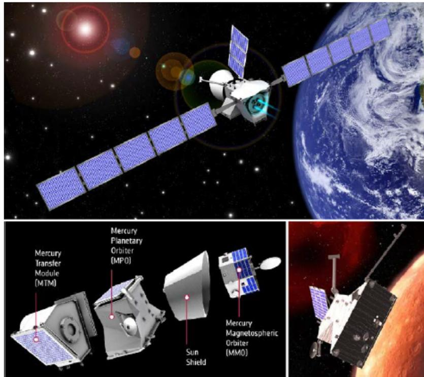
Figure 3.5: BepiColombo in cruise (top), exploded view during cruise (bottom left) and MPO at Mercury (bottom right) (credit: ESA)
