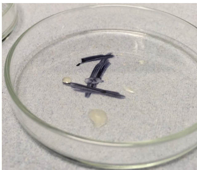
Figure 3.15: Discoloration of the IPA from the increased concentration of tars.
