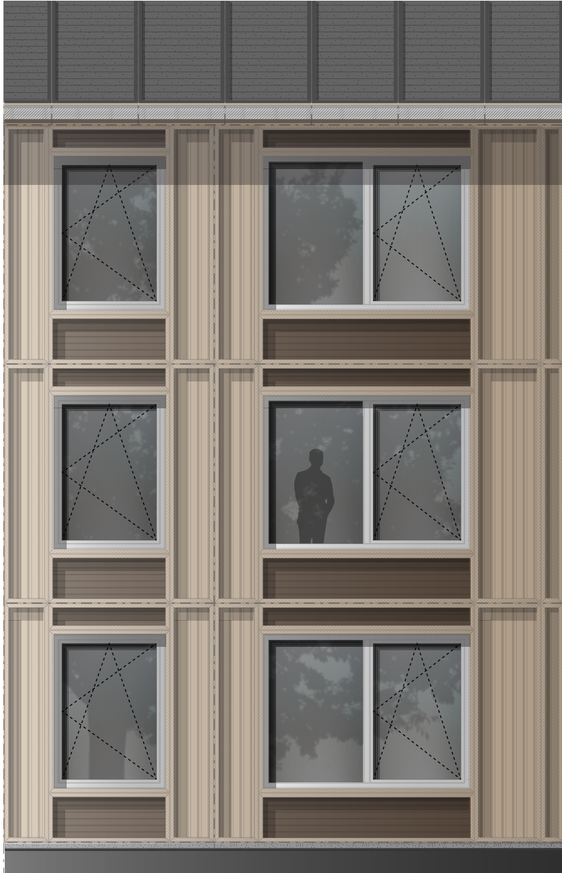
Fig. 9.5.4: Deeper extruded caps in combination with panel color variation (1:60) (own illustration)
