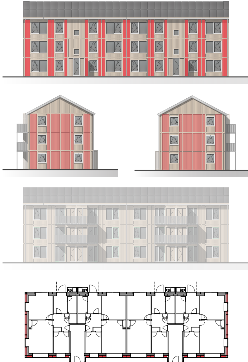
Fig. 9.4.9.2: (Top) The solar comb offers the best results on the south facade, alternatively the east and west facade could be utilised (own illustration).
