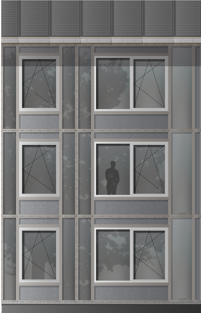
Fig. 9.5.8: Solar comb with glazing in front (1:60) (own illustration).
