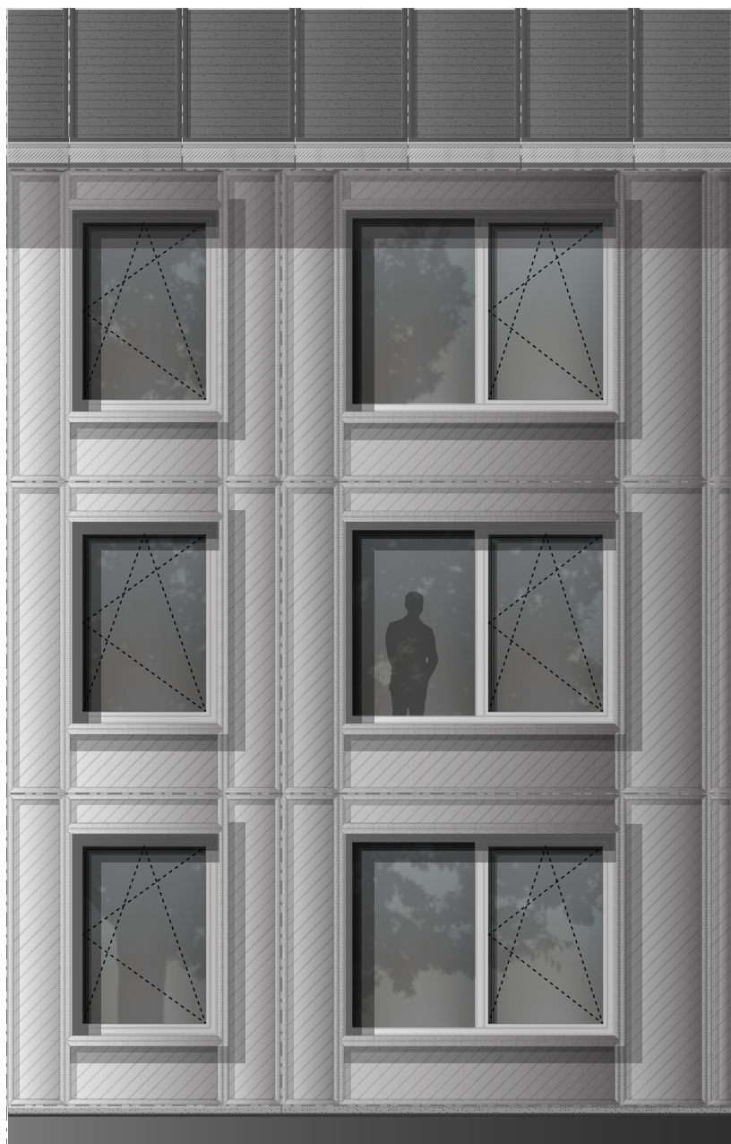
Fig. 9.5.6: Extruded static solar shading in combination with a steel finish (1:60) (own illustration)
