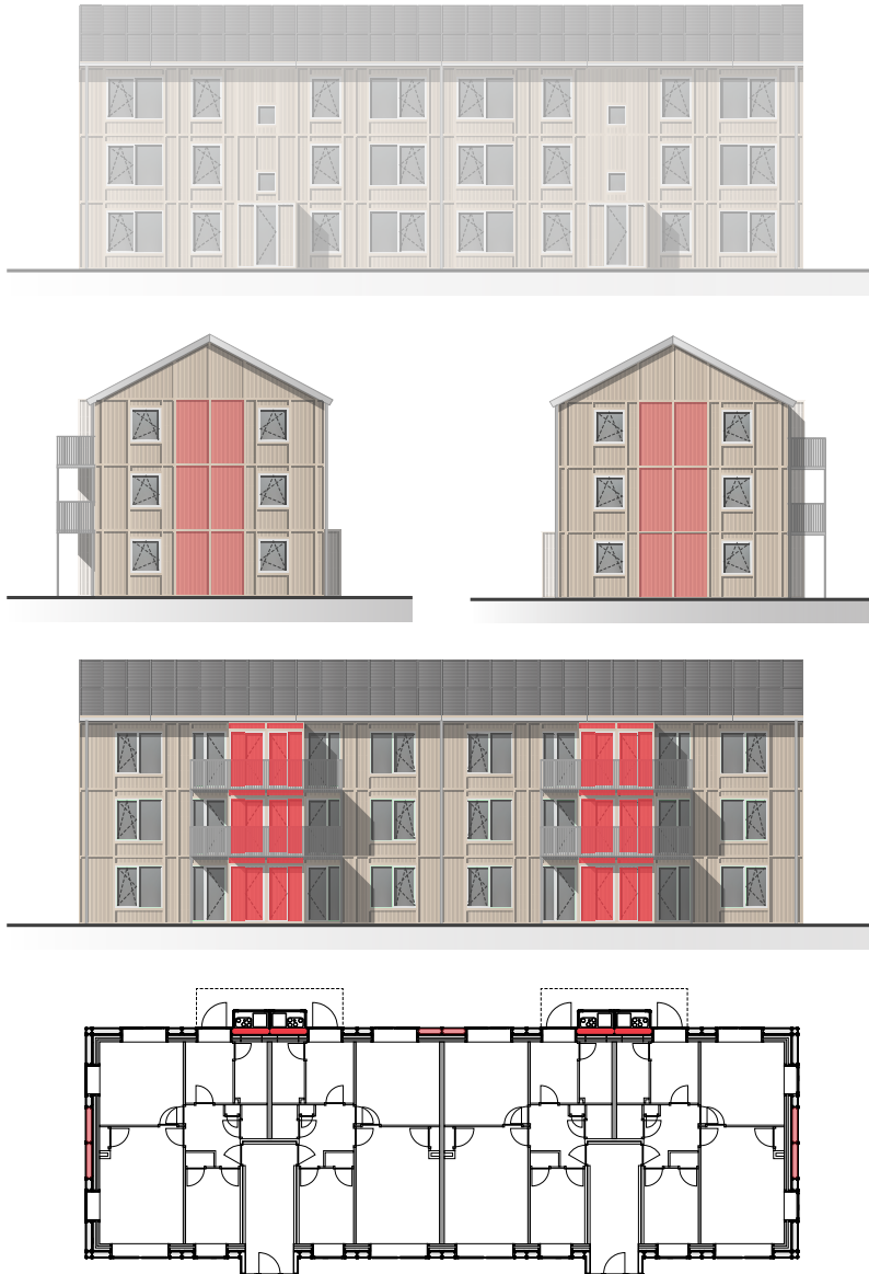
Fig. 9.4.2.3: (Top) The south and west facade could be used as potential alternative location for the installation box (own illustration).
