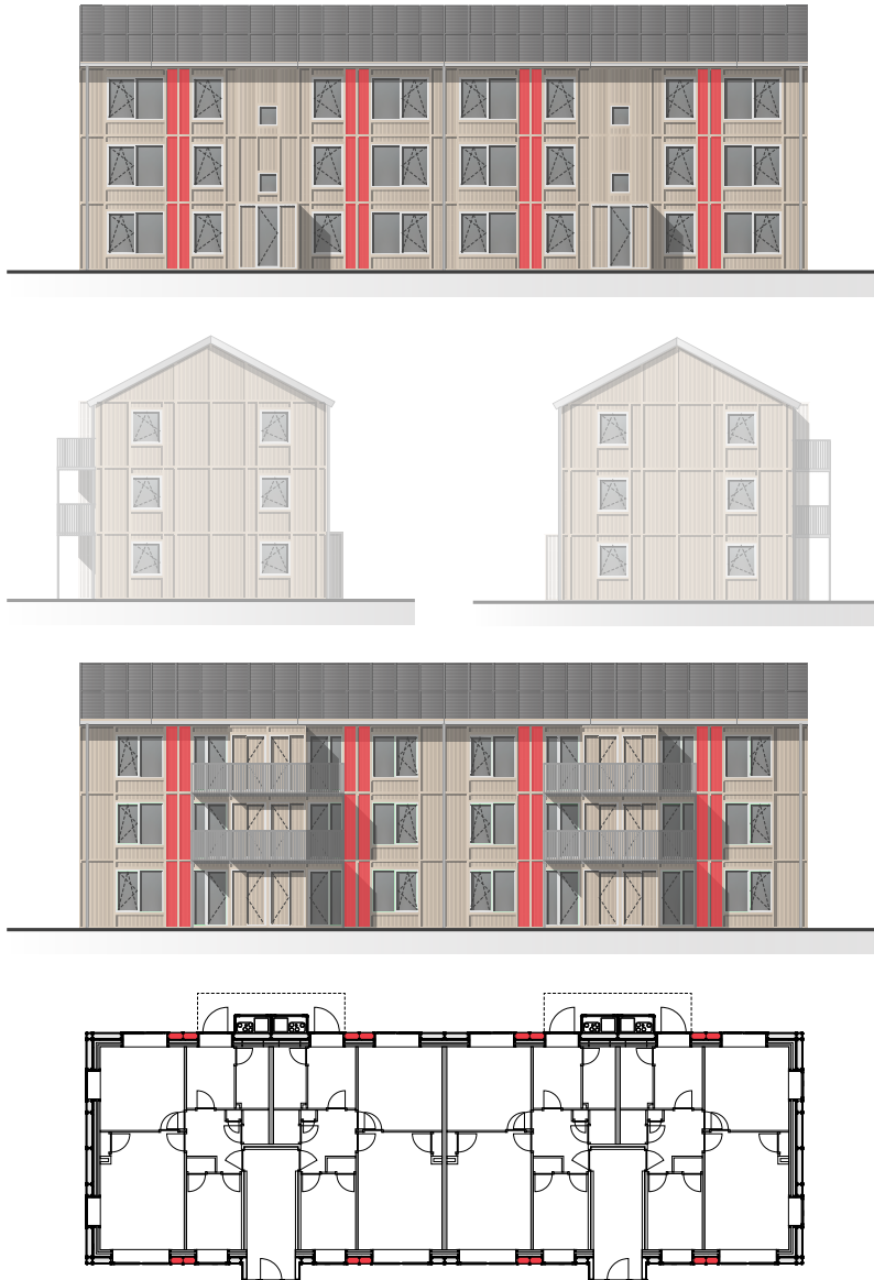
Fig. 9.4.3.3: (Top) Possible location boxes with integrated piping (own illustration).
