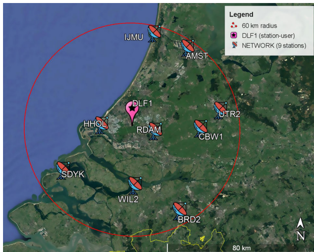
Fig. 5 Example of regional network for GPS dual-frequency (L1–L2) data retrieved on DOY 293 (in 2020). The nine stations are located within 60 km (circle) from a certain station-user
