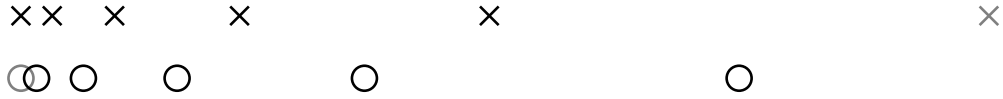
Figure 10. Illustration of primary (crosses) and dual (circles) grid nodes of an optimal/Krein grid for a semi-infinite-domain. The grid steps become progressively large as we move away from the measurement point, which coincides with the left-most primary grid node.
