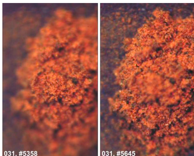
Figure 8. Material pile on the strong magnet: The two end-members of a through focus series of four images (sol 31, 5358, 5454, 5549, 5645). Both images shown are 1 mm wide (256 raw pixels). (left) Only the central top part of the pile is in focus. (right) The substrate surface is nearly in focus. The depth of field is 50\ \mu\text{m} and the sample wheel has been moved by 225\ \mu\text{m} (900 steps) toward the OM in between the acquisition of these images. These numbers imply a pile height of \sim 300\ \mu\text{m} , a rather common value for Phoenix soil material collected on the strong magnet.
