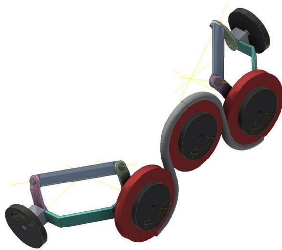
**Figure 10:** Combination between differential mechanism H1 with remote center of rotation B3.
