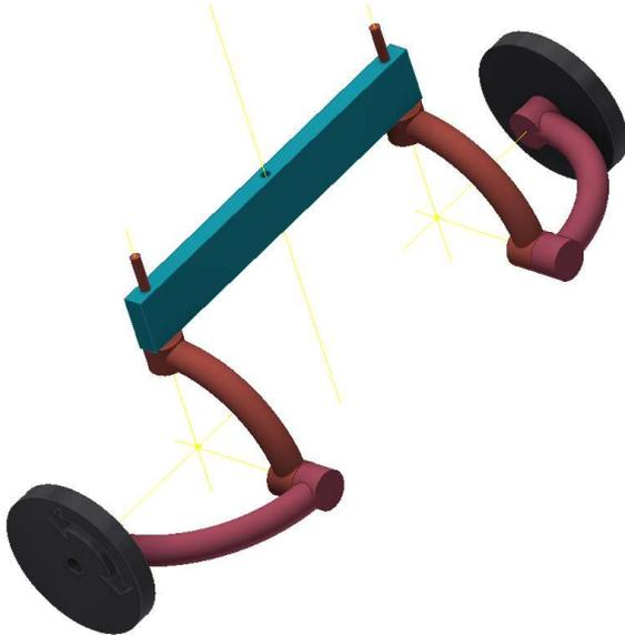
**Figure 9:** Combination between differential mechanism D2 with remote center of rotation H3.
