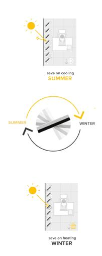
Figure 3.25: Scheme of the mechanism of Kindow. (www.kindowblinds.com)
