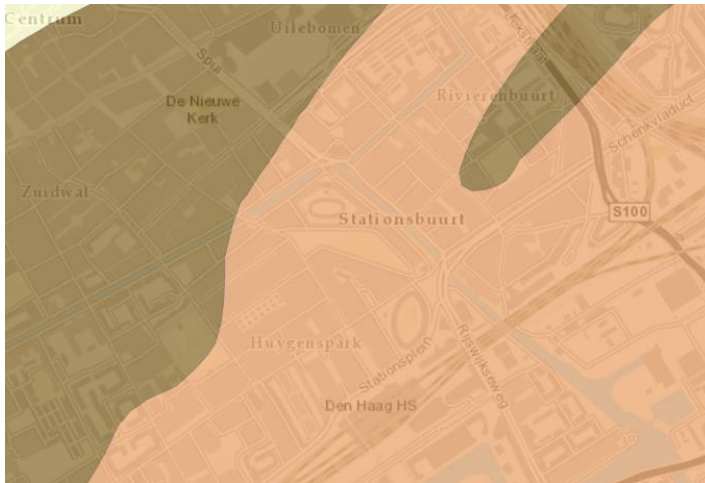
Figure 41: Geohydrological map of the Huygenspark (Gemeente Den Haag, 2021). Both colours show peat ('Hollandveen') on top of a sand layer ('Laagpakket van Wormer'). For the lighter colour, this sand layer is less than 5 metres below the surface.
