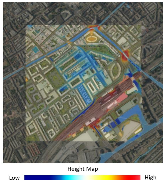
Figure 23: Height map of the Huygenspark with a colour scale from low (blue) to high (red) with an approximate range of +2.7 metres to -0.8 metres
