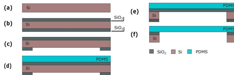
**Figure 3.** Process flow for the product platform: (a) Si wafer; (b) PECVD  $\text{SiO}_2$  deposition; (c) Back  $\text{SiO}_2$  patterning; (d) PDMS deposition; (e) DRIE Si etching; (f) Wet  $\text{SiO}_2$  etching. Figures are not to scale.
