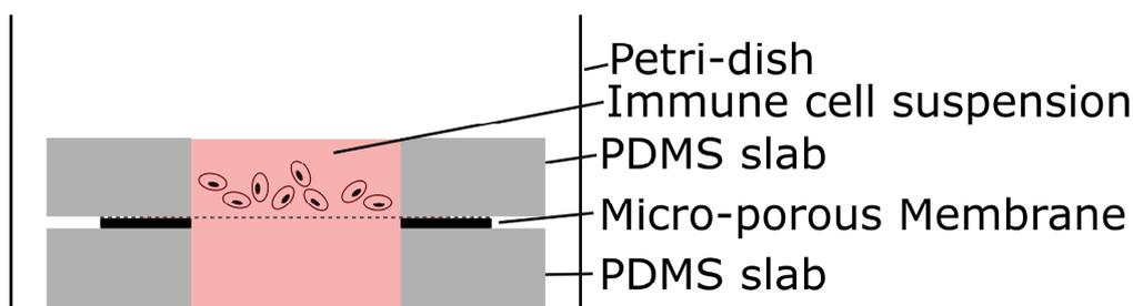
**Figure 5.** Schematic of setup for simple migration experiment.
