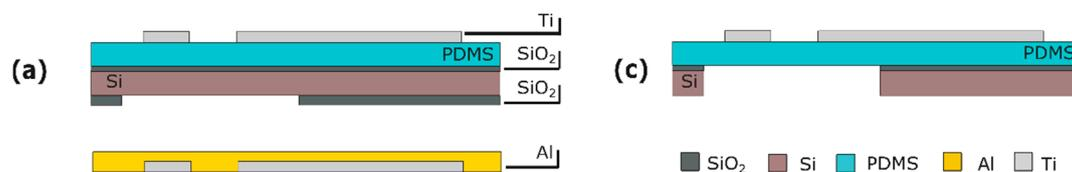
**Figure 13.** Process flow for the strain gauges: (a) Ti deposition and patterning; (b) Al deposition; (c) membrane releasing and Al etching. The figures are not to scale.
