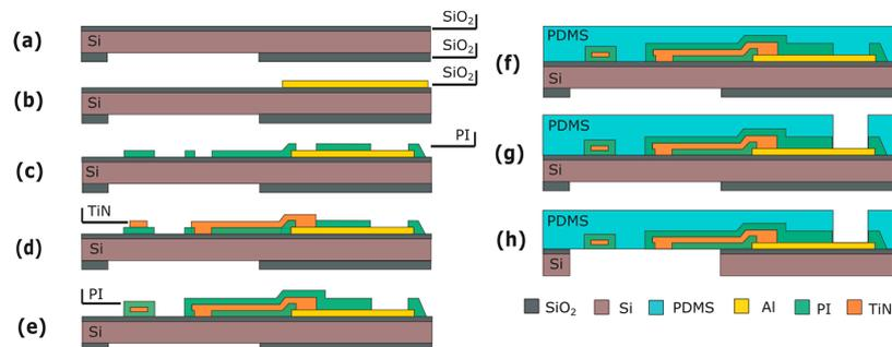
**Figure 8.** Process flow for the MEA module: (a) Substrate; (b) Al deposition and patterning; (c) First layer of polyimide (or, alternatively, parylene) is spun and patterned; (d) TiN deposition and patterning; (e) Second layer of polyimide (or, alternatively, parylene) is spun and patterned; (f) PDMS deposition; (g) PDMS patterning; (h) Membrane releasing. Figures are not to scale.
