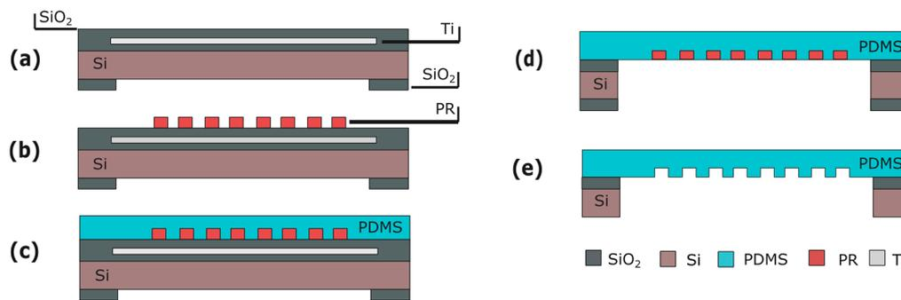
**Figure 11.** Process flow for the micro-groove module: (a) Substrate with Ti mask embedded in the front-side  $\text{SiO}_2$  layer; (b) PR spinning and patterning; (c) PDMS patterning; (d) Membrane releasing; (e) PR stripping. Figures are not to scale.
