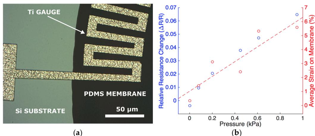
**Figure 15.** (a) Optical image from the front side showing a close-up of the Ti gauges at the interface between the silicon substrate and the PDMS membrane. As presented in [33], the strain gauges were fabricated on circular membranes; (b) Relative resistance change of a strain gauge (primary Y axis) and the average strain on the membrane (secondary Y-axis) as function of pressure.
