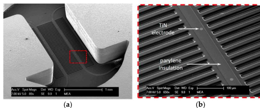
**Figure 9.** (a) SEM image of the Cytostretch chip from the back; (b) Close-up of the area highlighted in (a) depicting transversal micro-grooves, the exposed TiN electrodes and parylene insulation of the metal tracks. Adapted from [25].
