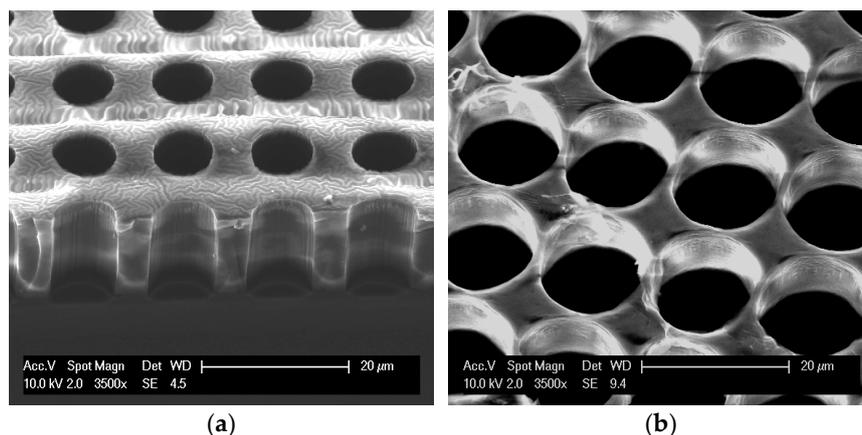
**Figure 6.** SEM images of microporous PDMS membranes: (a) 15- $\mu\text{m}$ -thick membrane with through-membrane pores 8  $\mu\text{m}$  in diameter; (b) 9- $\mu\text{m}$ -thick membrane with through-membrane pores 14  $\mu\text{m}$  in diameter.
