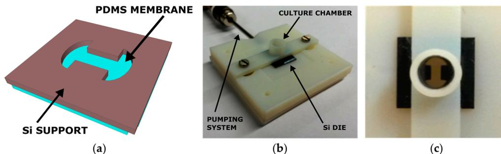
**Figure 1.** (a) Back view of the 3D sketch of the Cytostretch; (b) Example of a 3D-printed holder for the Cytostretch, including a cell culture chamber on top of the die and a pumping system to inflate the membrane; (c) Top view of the device mounted in the holder.
