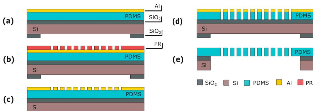
**Figure 4.** Process flow for the through-membrane micro-pore array: (a) Al sputtering; (b) PR spinning and patterning; (c) Al patterning; (d) PDMS patterning; (e) Membrane releasing. Figures are not to scale.
