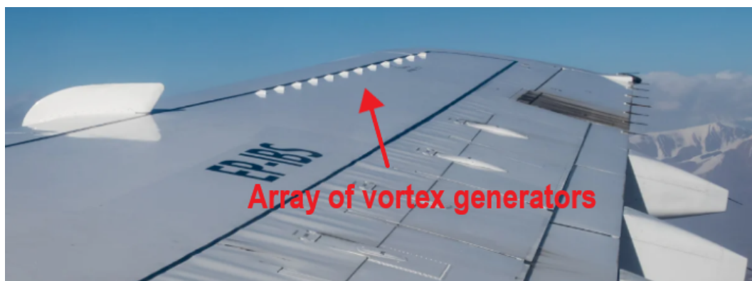
Fig. 1 Array of vortex generators on the outer wing of an Airbus A300B2 [17].
