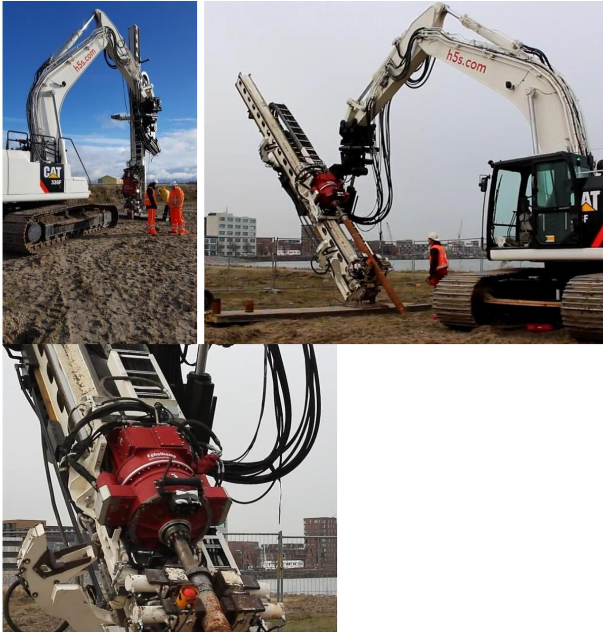
Figure K.1 Unit with sonic vibratory drill set.
