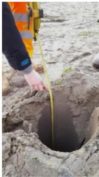
**Figure K.10 Measurement of settlement after retraction of the element**
