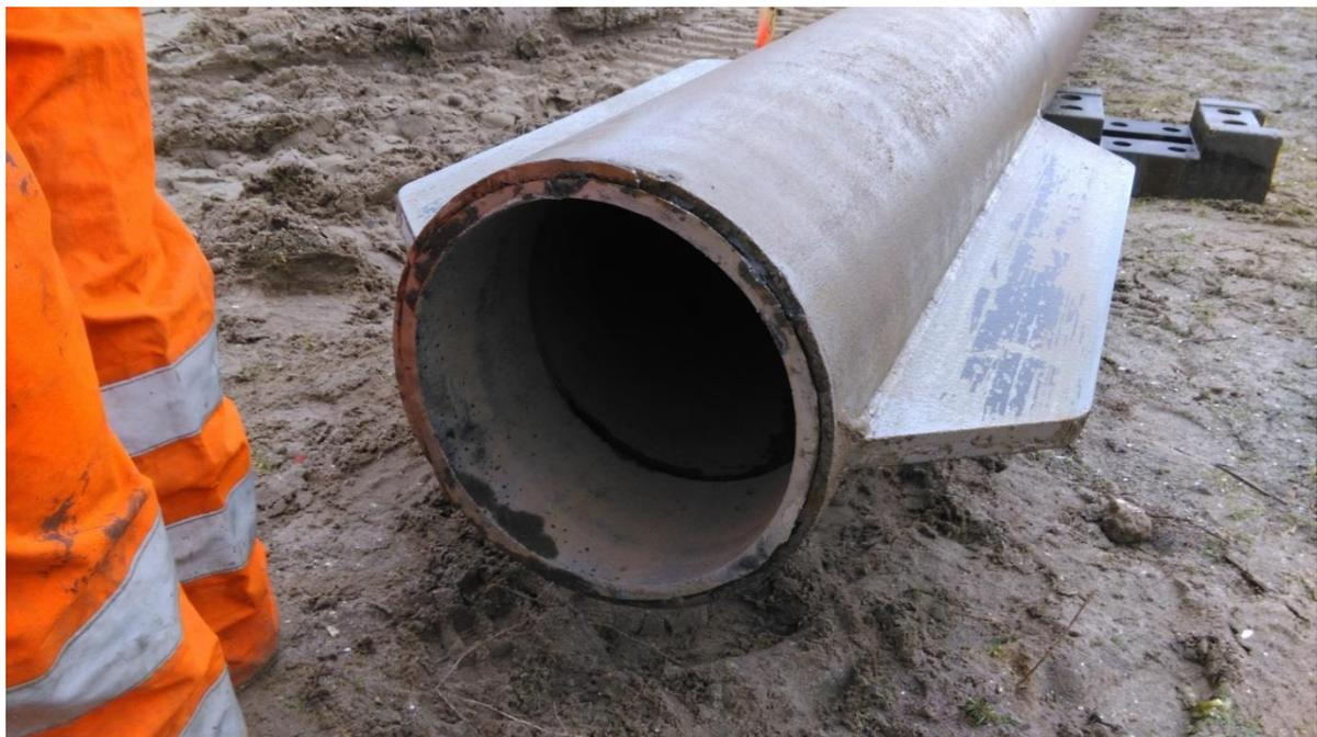
Figure 4.4 Open-ended element vibroflot shape 300mm
