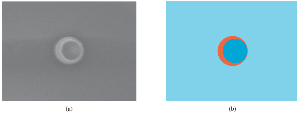
Fig. 16. (a) SEM image of a \text{SiO}_2 / Au composite nanoparticle. The silica nanosphere can be seen, as well as a the gold part on the left of the sphere, as a result of the etching from the right side and (b) a schematic representation of the particle as seen from above.
