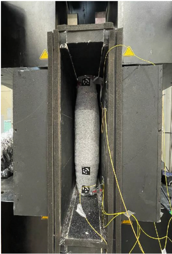
Fig. 1. Mechanical test set up of the wrapped composite joints.
