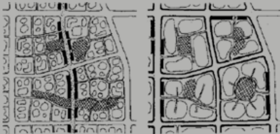
Figure 5. Two possible clusters designs with their public space. Black is commercial area, hatched is public space or park. Left: Few buildings are clustered together along a main street with public facilities, with publicly accessible parks and squares. Right: Blocks are clustered with semi-public parks and squares and public facilities around the borders (Miao, 2010).
