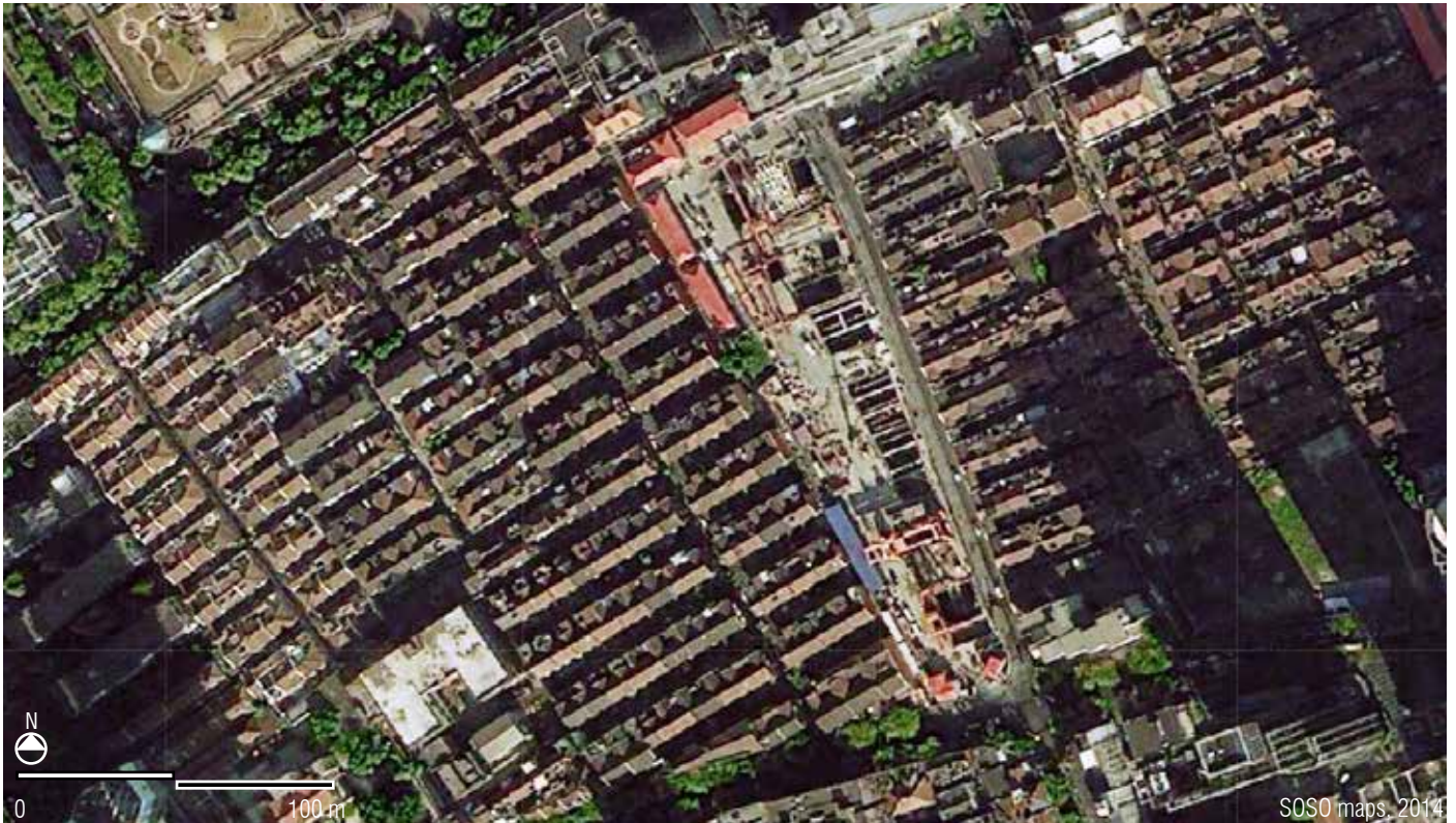
Figure 136. Lilong housing in Shanghai has a very high population density due to the large number of families sharing the dwelling units. The FAR is low as houses are not very tall. In general, Lilong dwellings have two or three storeys.
