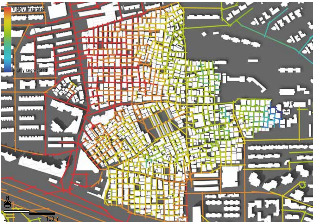
Figure 172. Axial Step Depth. From the main street, almost the entire urban village is accessible through the implementation of the new network. No segregated areas exist.
