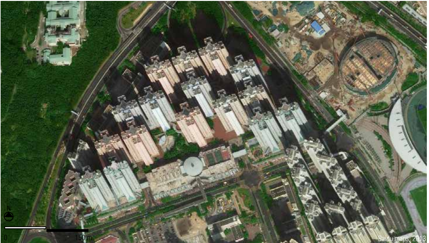
Figure 132. High-rise residential plan in Hong Kong has a very high FAR due to buildings with many storeys on the plot. This results in many inhabitants and much space per person.
