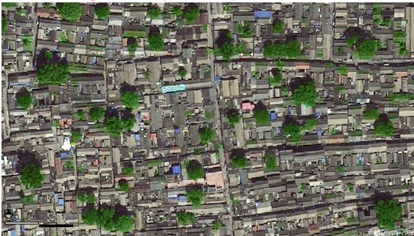
Figure 135. The traditional Hutongs in Beijing consist of one or two storey courtyard houses. The density is high, because multiple families live together in one dwelling unit. Therefore the FAR and amount of space per person is low.
