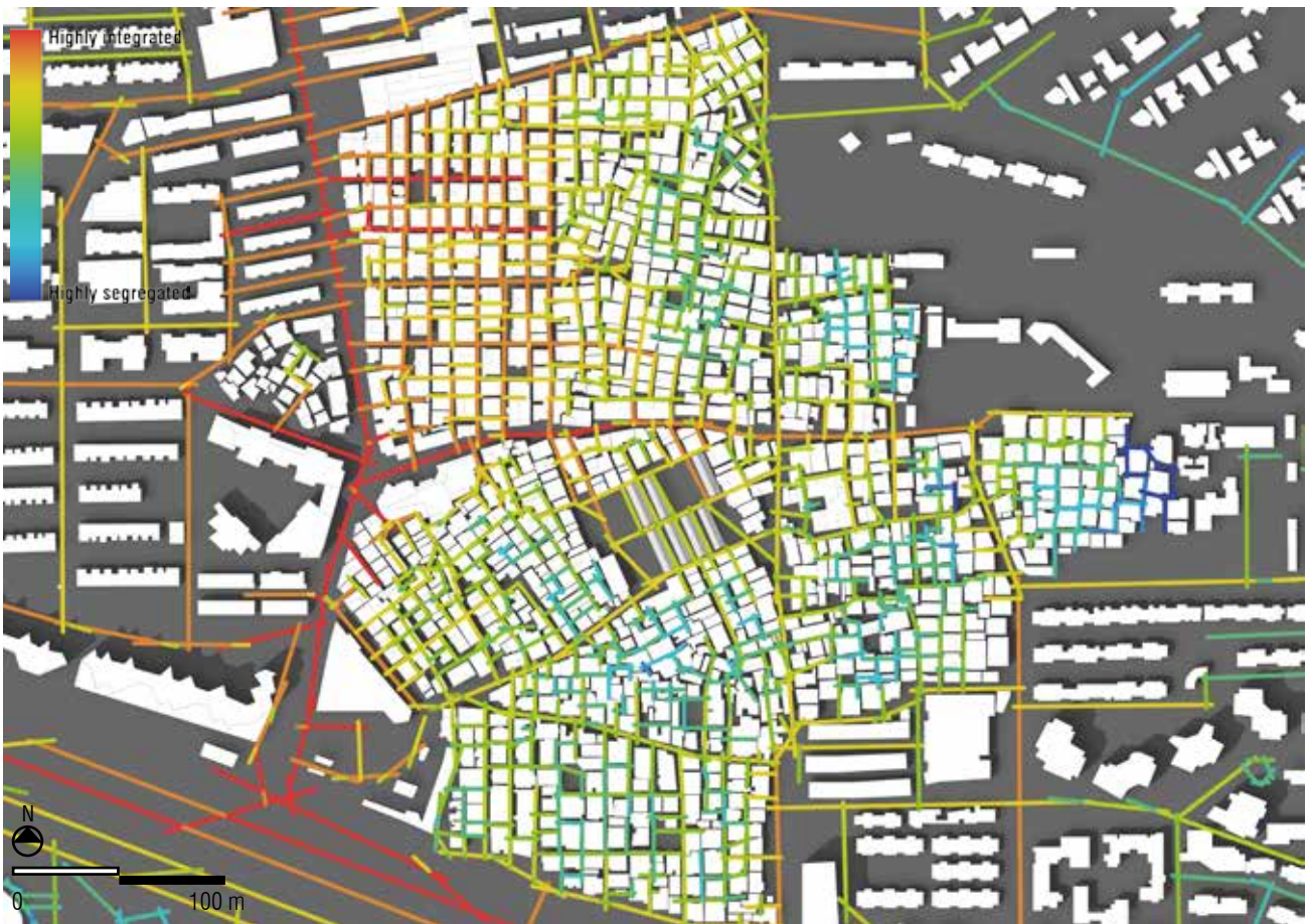
Figure 174. Angular Step Depth - LOCAL PASSERS -. One of the most important aspects is to incorporate inhabitants from gated communities. The areas indicated in red, orange and yellow show high level of integration.
