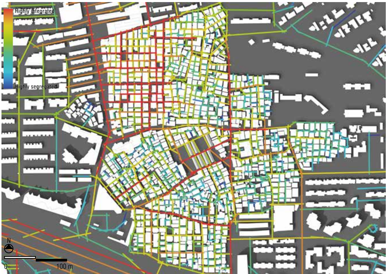
Figure 170. Local Integration [R3]. In the current situation only the main routes within the neighbourhood are coloured red. With the new network structure, several streets are locally much more integrated and therefore more accessible.
