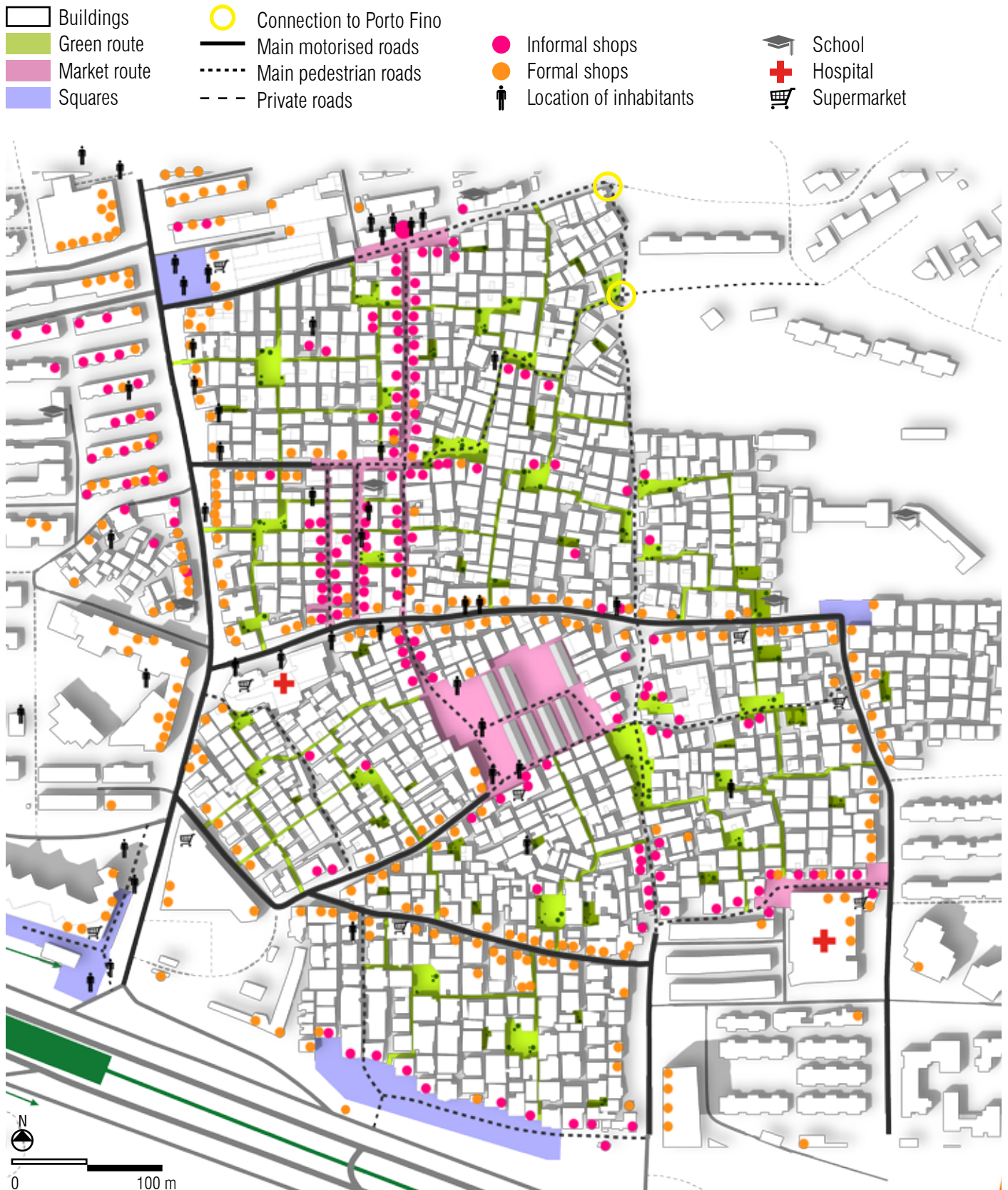
Figure 168. Main vehicle routes will be upgraded and an additional pedestrian route will be introduced to connected to Porto Fino. The positioning of these routes is based on the availability of current formal and informal facilities and Space Syntax analyses. An additional green route will be implemented to downsize the large neighbourhood.
