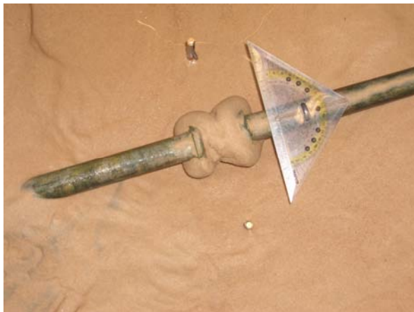
Figure 6-15 Top view, result of test 2: low injection rate, compaction grouting
