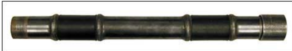
Figure 5-8 Injection system used in practice (diameter = 60mm).
