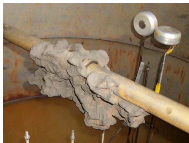
Figure 6-31 Side view of the grout fracture
