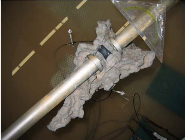
Figure 6-41 Excavated grout fracture in test 9
