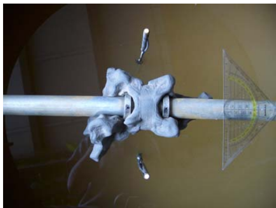
Figure 6-26 Top view excavated grout fracture in Test 5. The Rubber sleeve closes after injection
