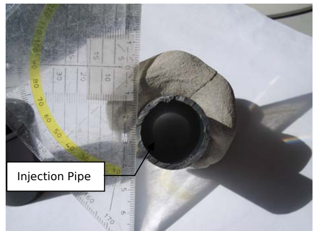
Figure 6-16 Side view of hardened grout injection of test 2 (excavated and detached from the injection pipe)
