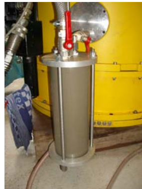
Figure 5-22 Bladder filled with grout
