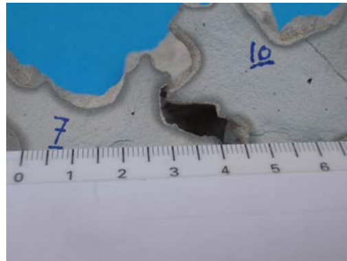
Figure 7-3 Test 7 and 10 bleeding layer (cross sections of the fracture)
