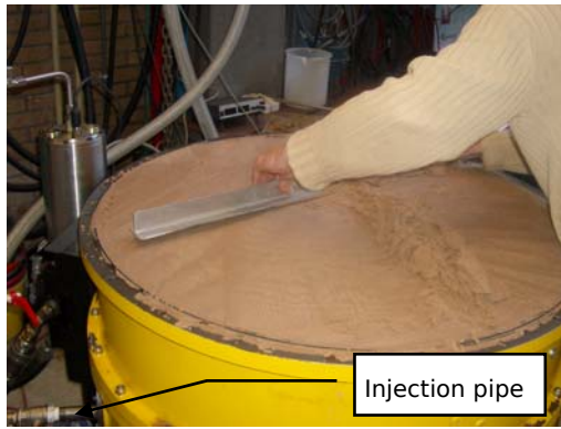
Figure 5-13 Flattening the sand surface
