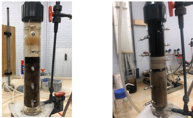
Figure 6.2.1: Performance of the mixture installed under water (left) and after a current from below the layer (right)
