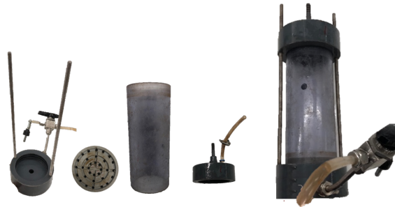
Figure 3.3.3: Components of the columns. From left to right: Cells with two metal rods (1), the plastic porous cylinder plate (2), the transparent plastic cylinder (3) and the lid that can be connected to the standpipes (4).
