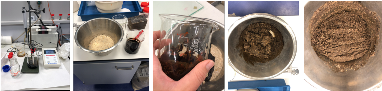
Figure 3.3.1: Visualisation of different steps of mixing of flocs in the sand. From left to right: Making the flocs, the floc mixture and the clean, dry sand, pouring the solution over the sand, halfway through the mixing, the mixed Al-OM-sand.
