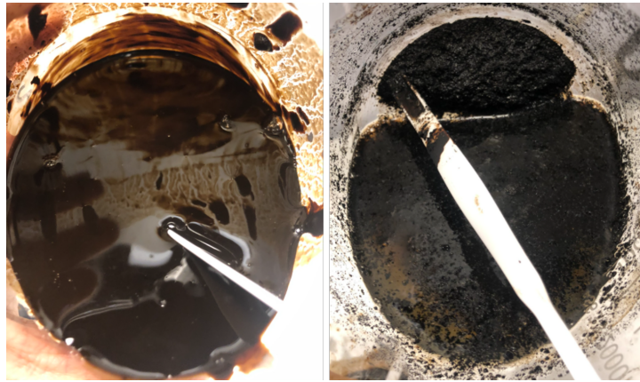
Figure 5.2.1: Floc solution obtained by mixing Al and OM in solution (left) and the floc solution obtained by mixing Al and OM in powder form (right). As shown, the flocs produced by mixing in solution has the shear-dependency feature, while dry mixing created particles that have a constant size.
