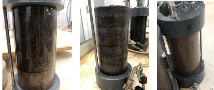
Figure 5.2.3: Columns that show heterogeneity in the sample due to separation of flocs from the sand during compaction.
