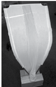
Figure 6.52. Scale model (1:3.5) of canopy, showing frame and counterweights and blue textile permeable air duct mounted on top
