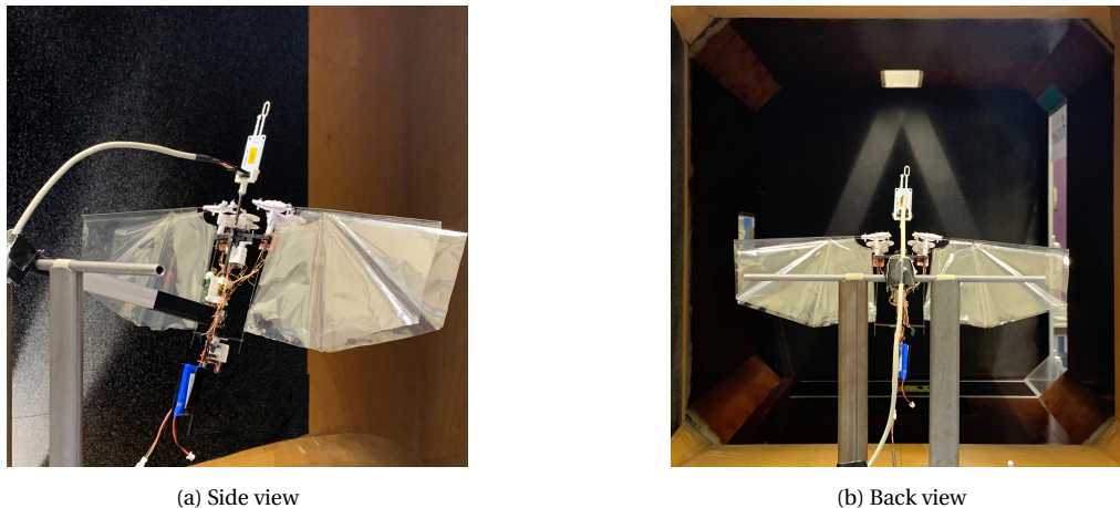
Figure 3.15: Delfly being clamped onto a custom-made W-tunnel support structure for fixed flapping tests, placed at the exit of the 60 \times 60 \text{ cm}^2 contraction section.
