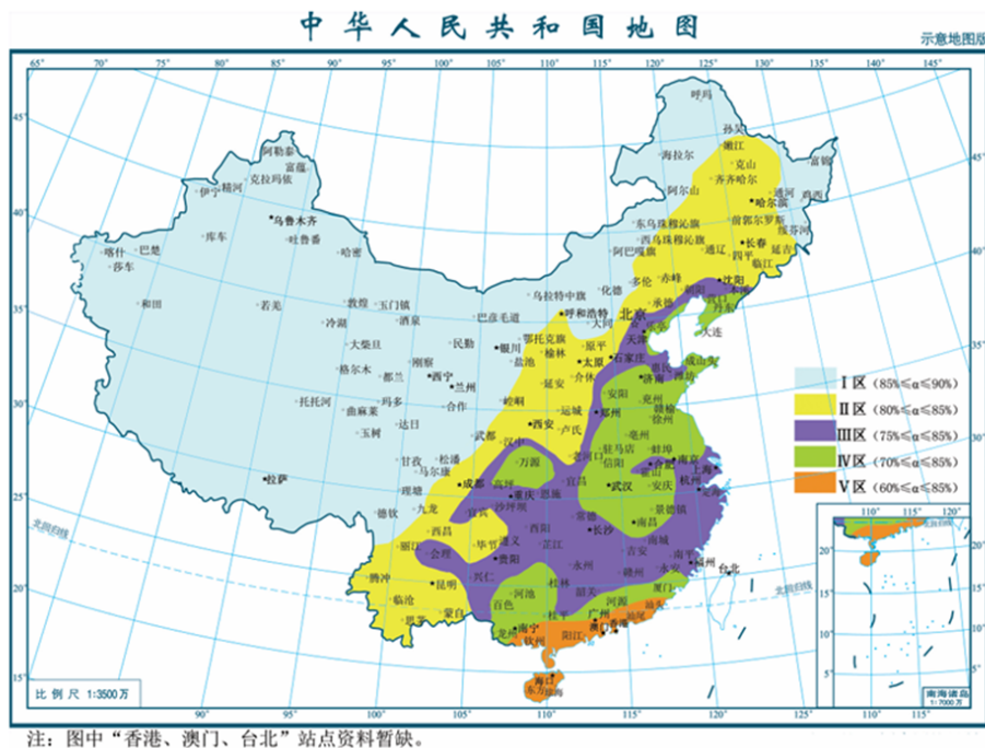
Figure 4.5: Zoning map of total annual runoff control rates for the continental region of China, adopted from Ministry of Housing and Urban-Rural Development (2014). Light blue: Zone I, light yellow: Zone II, purple: Zone III, green: Zone IV, orange: Zone V.
