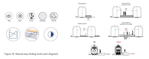
Figure 17. Platform dimensions (own diagram)
