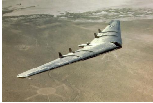
Figure 2-7 Northrop's flying wing concept: YB-49
