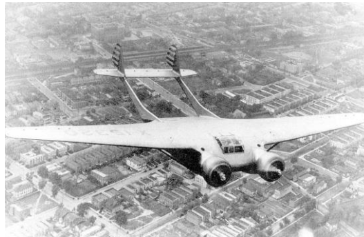
Figure 2-5 Burnelli's lifting fuselage configuration: UB-14
