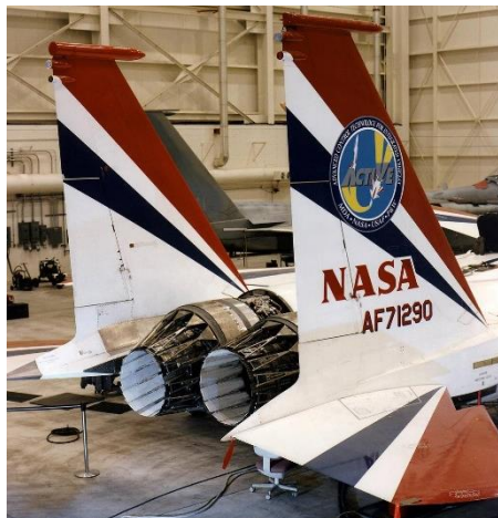
Figure 2-24 Type II vectoring nozzle, picture: NASA
