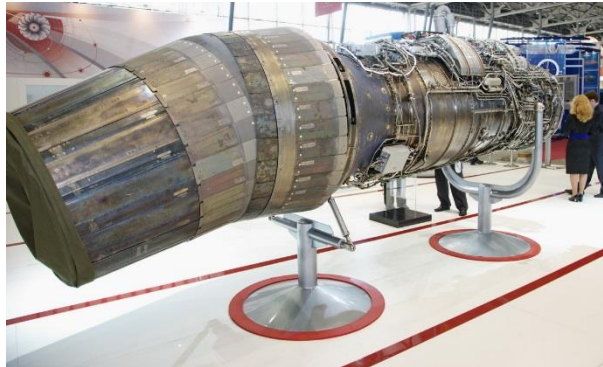
Figure 2-23 Type I vectoring nozzle, picture: NOP Saturn
