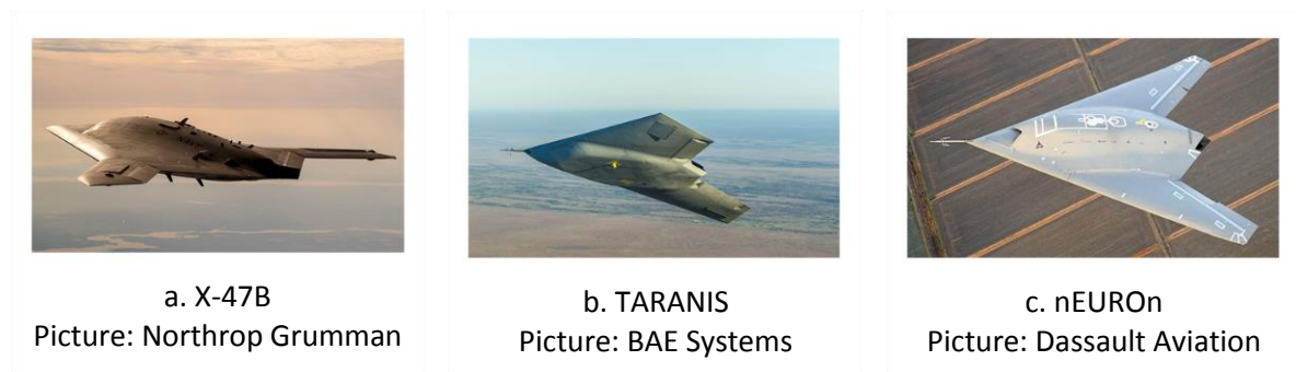
Figure 2-9 UCAV demonstrators with ALV configurations
