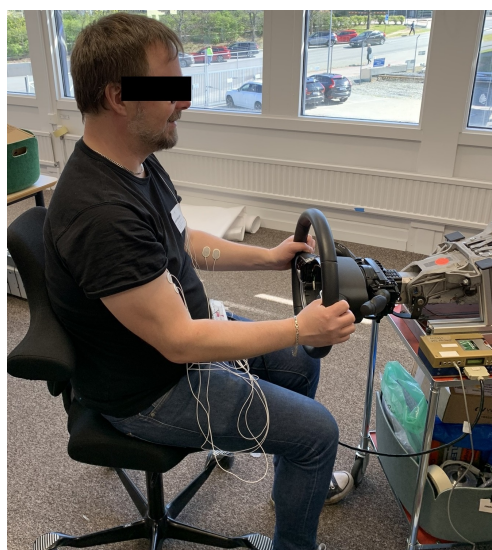
Figure 4. Participant holding the steer in quarter-to-three hand to steering wheel position.
