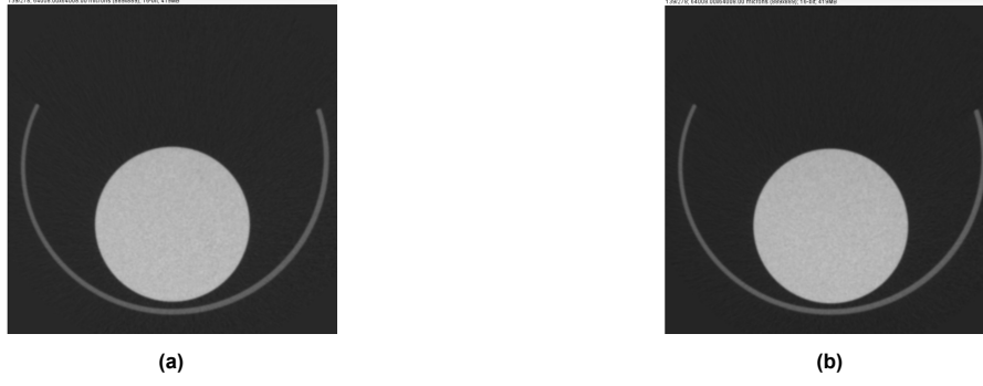
Figure C.2: Both images are the middle slice of the CT images of the trabecular bone. On the left side, the insert is scanned with 50 kV, and on the right side it is scanned with 55 kV.
