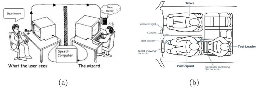
Figure 4. (a) shows a general WoO experimental setup (Harwood, 2018) and (b) shows a WoO setup in a TTS experimental setup (Ekman et al., 2016).
