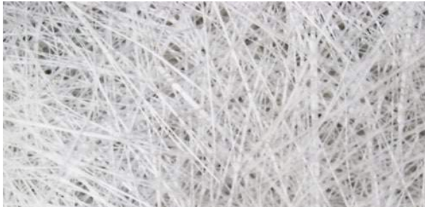
2.15 Random orientation in glass fibre chopped strand mat ( http://tienda.resineco.com/en/VI00005 )
