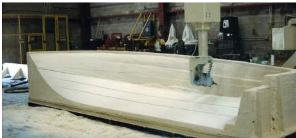
6.18 Foam shaped by a CNC router for a boat hull mold ( http://www.reinforcedplastics.com/ )
