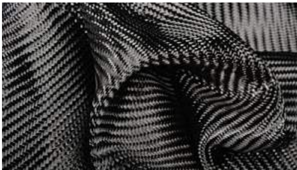
2.4 Fabric woven with carbon fibres in twill weave. ( http://www.hccomposite.com/en/catalog/34/1969.html )
