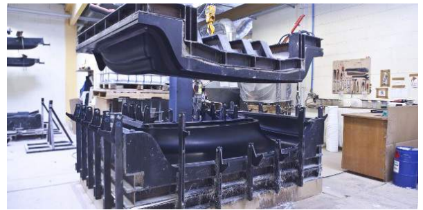
6.9 Double mold for resin transfer molding ( http://savercompositi.com/ )
