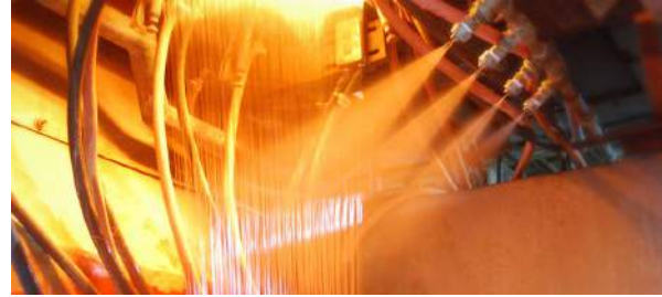
3.10 Cooling down of molten glass filaments by water jets ( http://binaniindustries.com )
