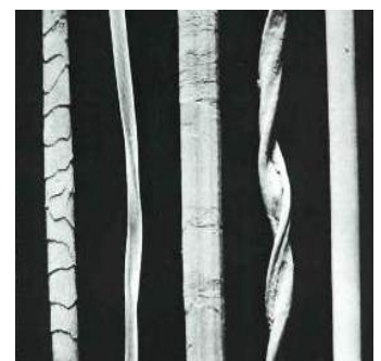
2.18 Fibres of cashmere, silk, linen, cotton and polyester from left to right. ( http://www.alpacasocksrock.com )
