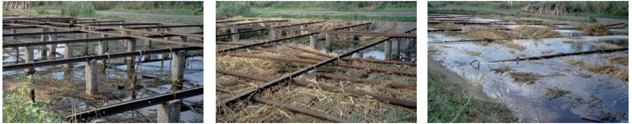
3.2 Processing of water retting in a concrete retting pool. The bales of hemp sheaves are placed in the pool and secured with metal bars. The pool is filled with water and the stems are let in to ret for 5 days. (Van der Werf, H. M., & Turunen, L.,2008)
