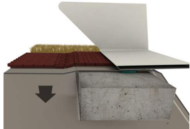
9.10 Soil compaction next to the foundation (concrete block solution)
