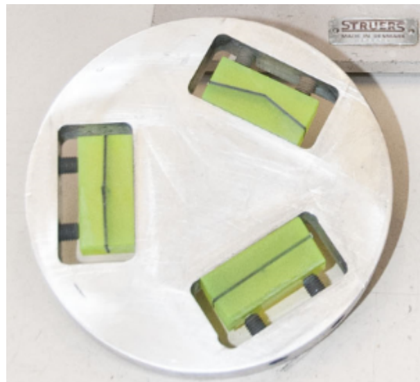
Figure 3.3: Sample after being ground and polished up to 1 \mu\text{m} .
