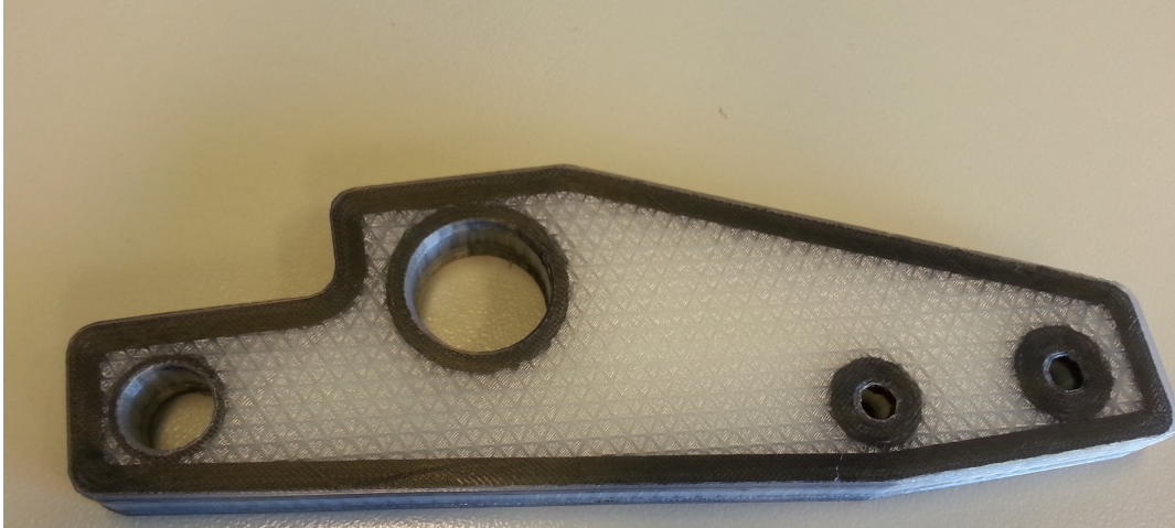
Figure 6.9: Final part as printed by the Mark Two ® . It can be seen that the bottom 30 and top 30 layers are reinforced. The costs of this part are 248 Euro.
