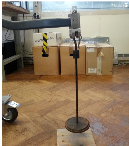
Figure 6.11: Complete test set-up. The weights can be stacked on the pendulum in order to increase the load on the bracket. A wooden board is placed under the pendulum to prevent any damage to the floor in case of failure.
