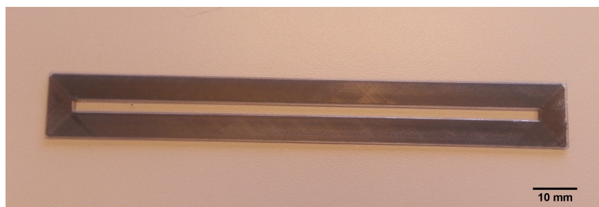
Figure 3.1: A completed sample by the Mark Two ® . The fibre bundles are placed concentric so that these are unidirectional in the long parts of the sample.
