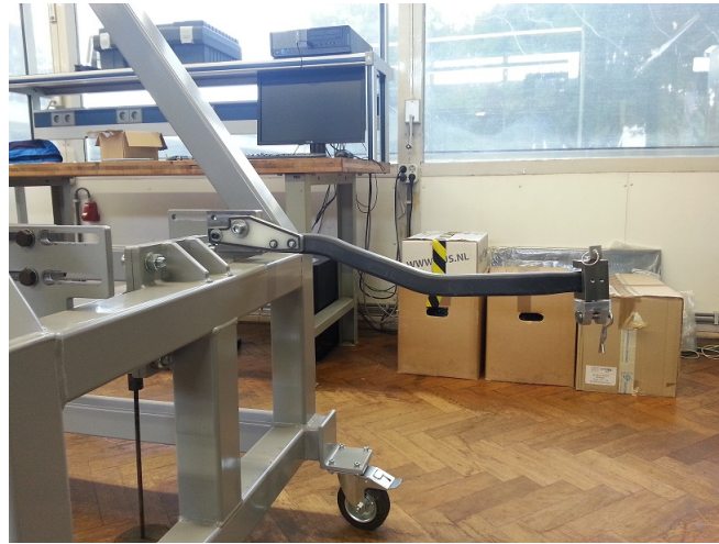
Figure 6.10: Test set-up for testing the 3D printed chair bracket. The bracket is mounted to a steel plate by two bolts. The metal part at the end of the arm is used to hang the load on.
