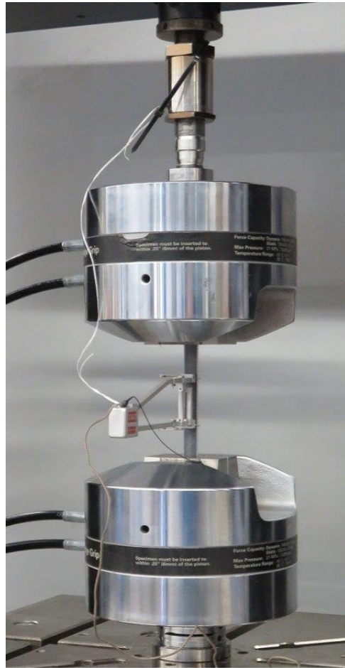
Figure 3.5: Initial test set-up of the ASTM D3039-14 tensile tests on the Instron ® 5900R tensile test machine. The coupon is placed between the two clamps and an extensometer was applied.
