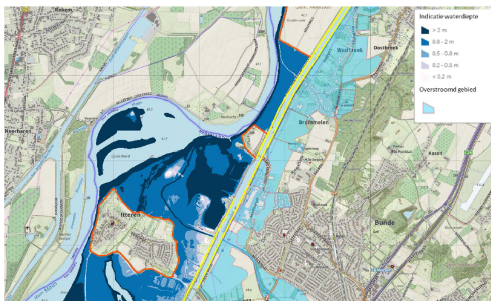
Figure 1.1: Estimation of the flooded area and water depths (ENW, 2021). The shades of dark blue indicate the water depths west of the canal, and the light blue indicates the flooded area east of the canal.
