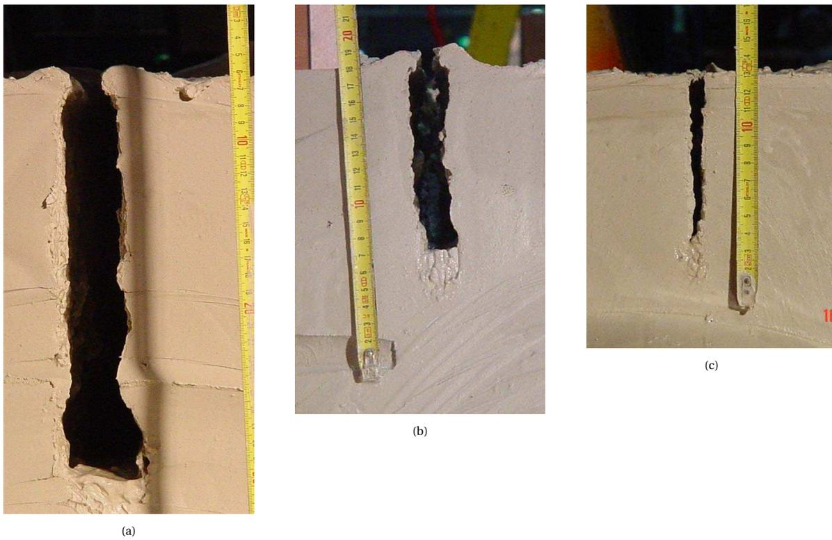
Figure 3.10: Typical cavity shape of a penetrating jet (Nobel, 2013)
