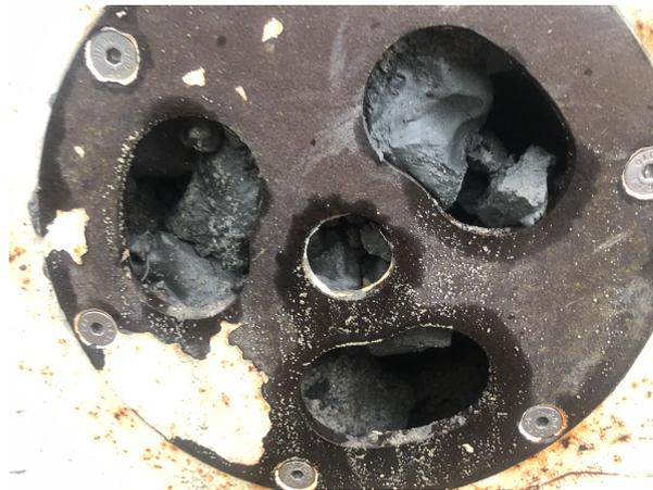
Figure 4.7: Clay blocks during jet trenching in clay (photo: DEME)
