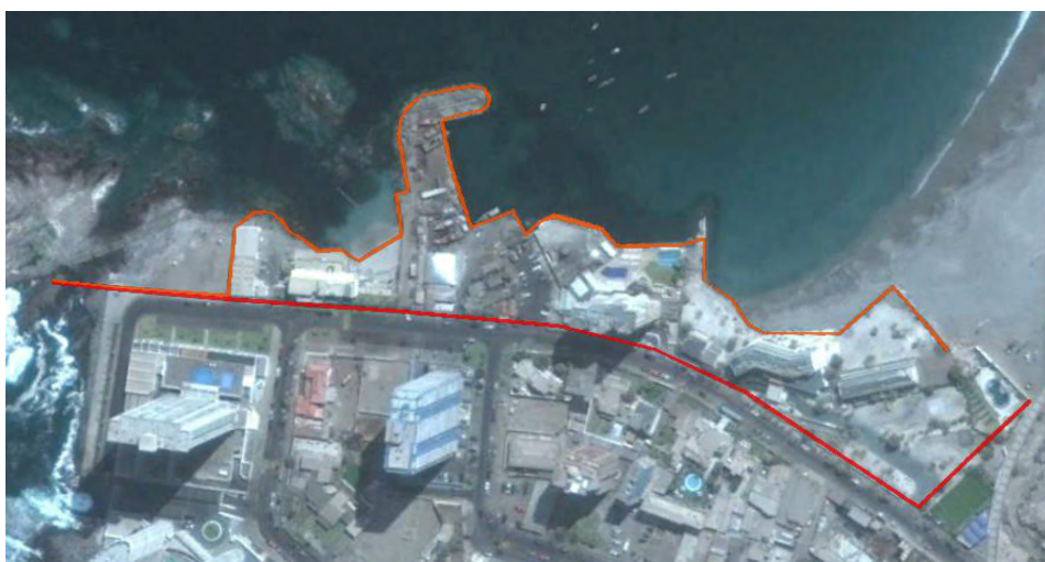
Figure 3.9: The two possible traces for a seawall in the north Cavanca region
