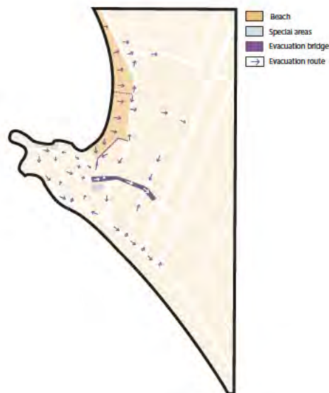
Figure 3.23: System option 2 - Horizontal evacuation (using bridges), Cavancha
