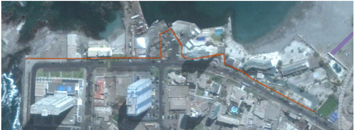
Figure 3.13: The final seawall trace is shown in orange. From this trace a raise from mean sea level of five meters can be realised. For this the wall height will vary between 2 and 3 meters. In purple the final Dyneema barrier trace is shown.
