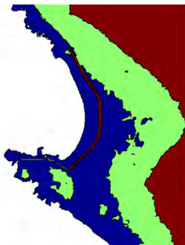
Figure 3.27: The implementation of the Dyneema barrier and the seawall in the grid. The contours of the 0, 5 and 10 meters are given in blue green and red respectively.
