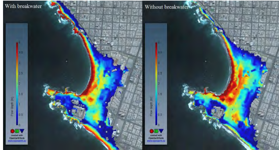
Figure J.7: Comparison of the inundation area in the case with and without submerged breakwater.
