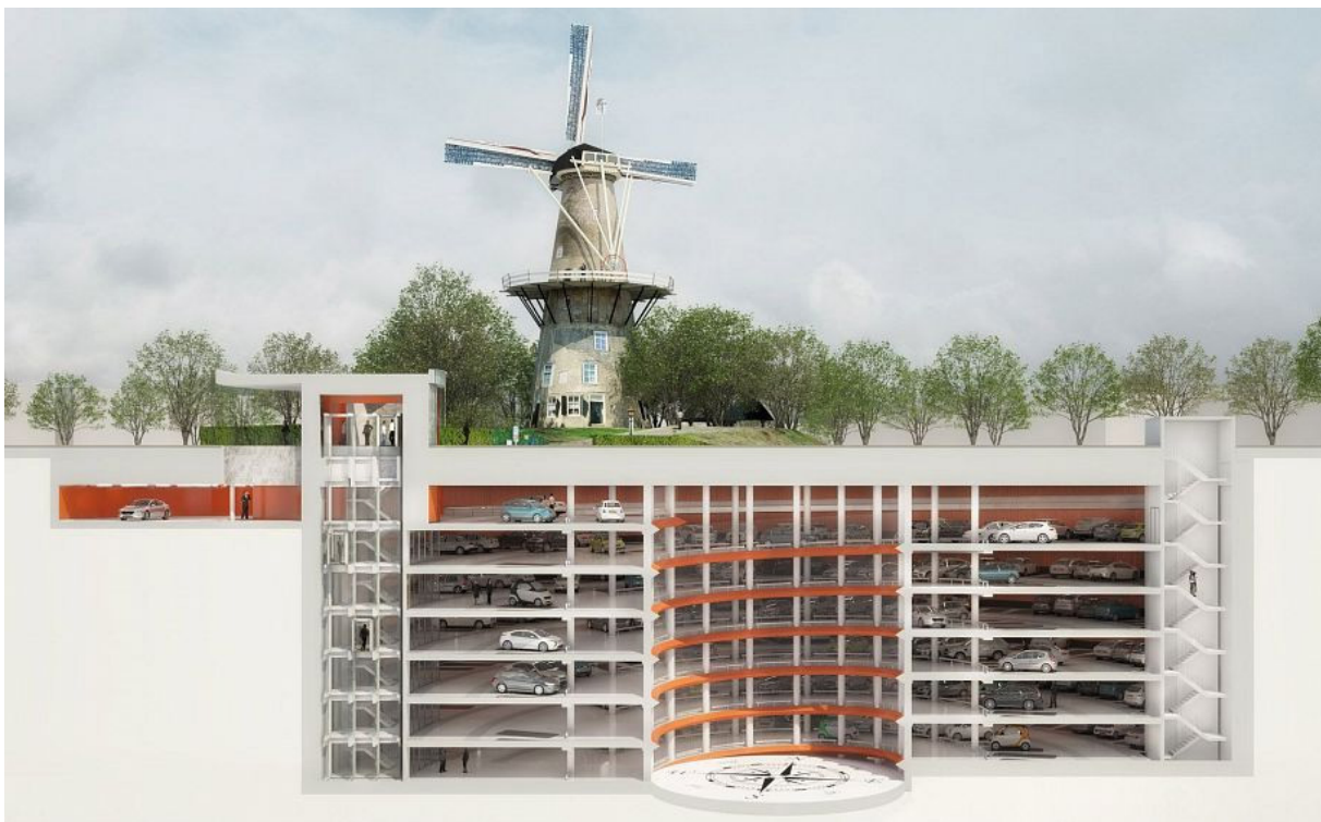
Figure 29: Section showing the depth of the car park with the central atrium
