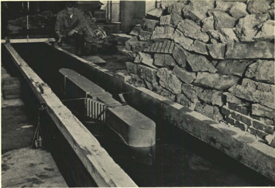
Fig. 4. Krachtmeting in Model A.
