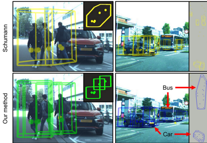
Fig. 9. Challenging cases for clustering, camera and top view. DBSCAN falsely split the car and the bus but merged the pedestrians into a single cluster, making Schumann [2] (top) fail. Our method (bottom) managed to classify the radar targets and cluster them correctly using class-specific parameters. Yellow marks other class.
