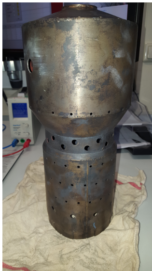
Figure 6.6: Discolouration pattern on the RQL liner
