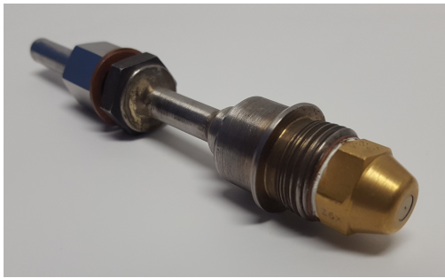
Figure 4.10: Fuel nozzle with its nozzle holder
