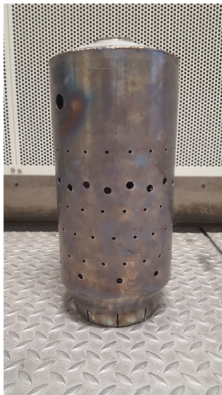
Figure 6.9: Discolouration pattern on the RQL liner
