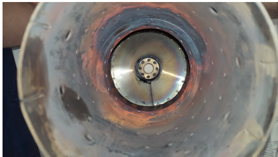
Figure 6.7: Inside of the RQL liner
