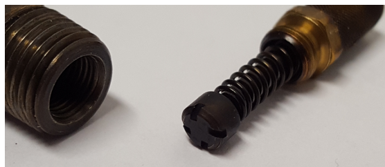
Figure 4.8: Insides of the pressure swirl atomizer used
