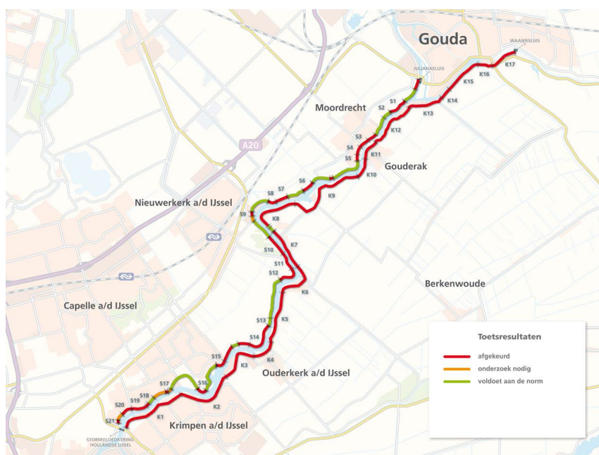
Figure 2.2: Results of third test round 2011. Insufficient dikes are coloured red. Source: Kraaijenbrink (2010).
