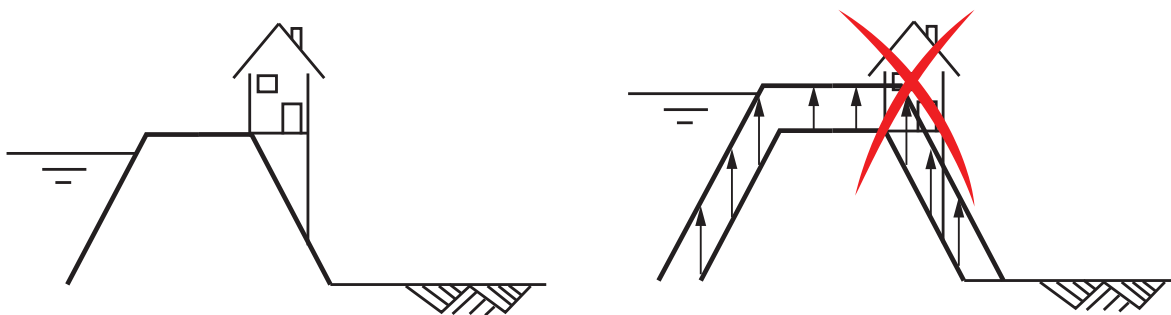
Figure 6.13: Option 7: Removal of a building due to dike reinforcement near a building.
