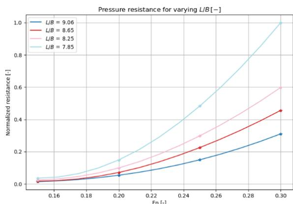
Figure 7-8: Pressure resistance for various L/B-ratios.
