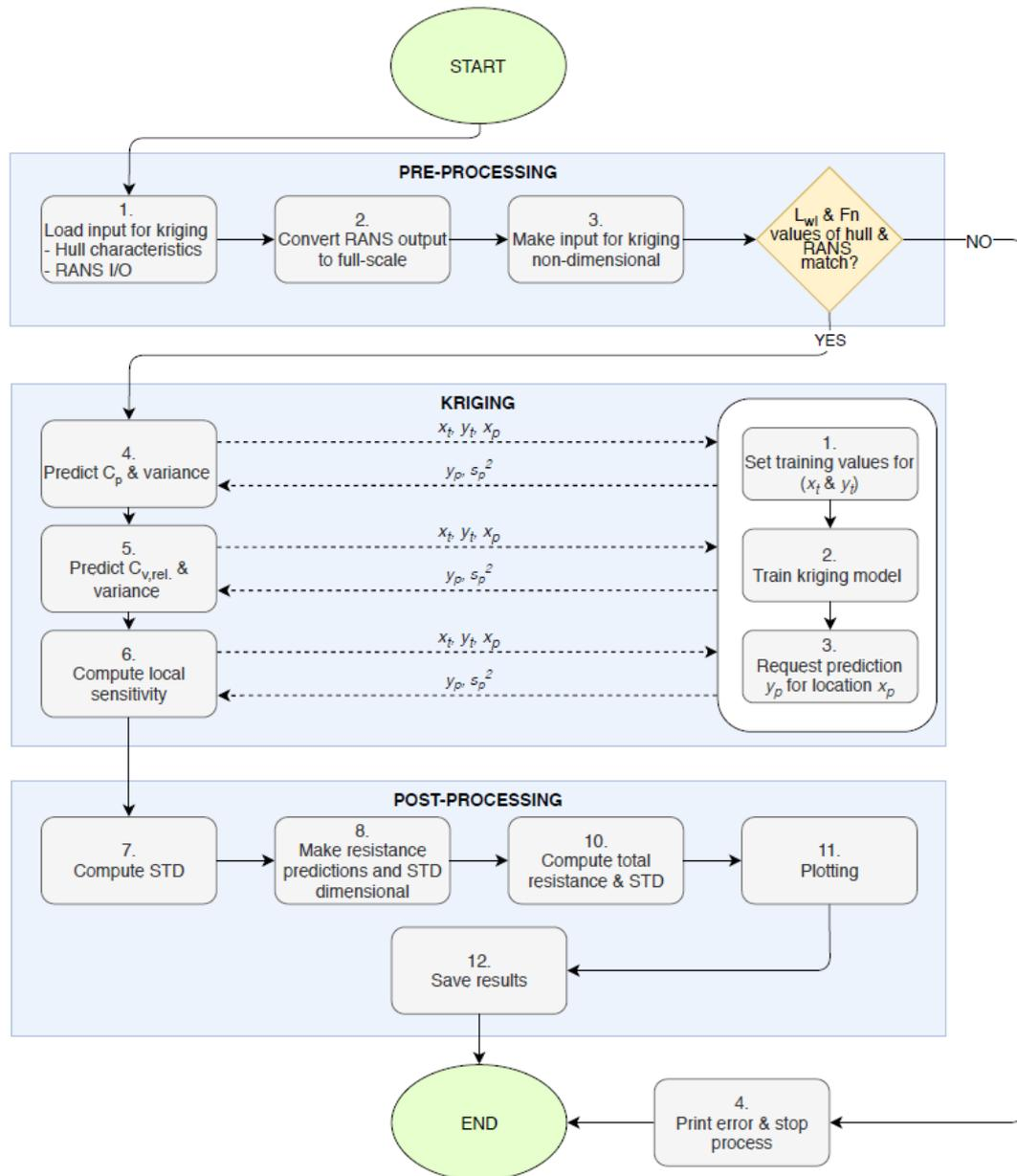
Figure 5-8: Low-level overview of the kriging procedure.
