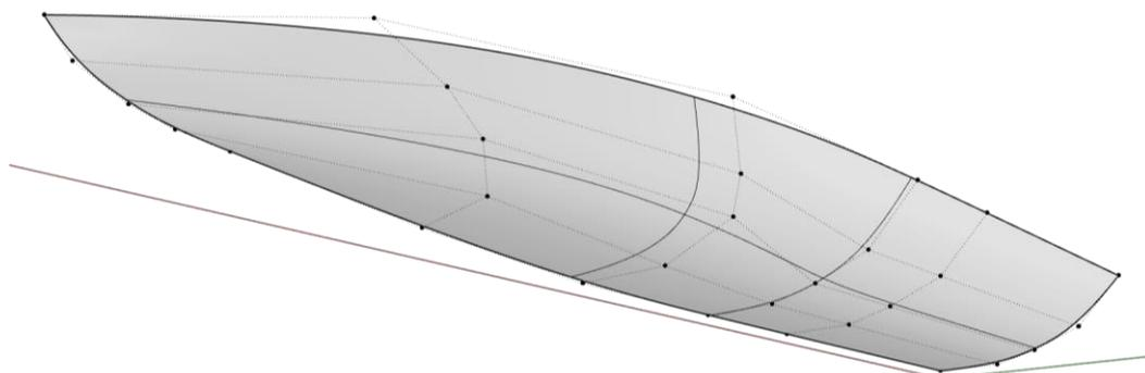
Figure 5-3: One quarter of the base hull with control points visible.
