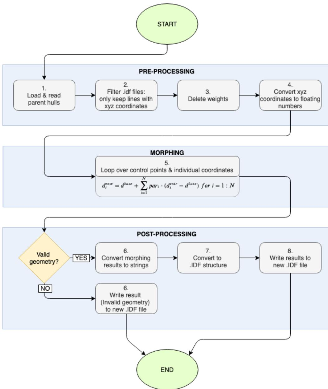
Figure 5-2: Low-level overview of the morphing procedure.
