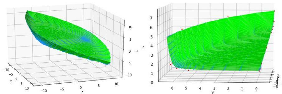
Figure 7-3: Geometry of the selected hull with control points concentrated near the mid-ship.
