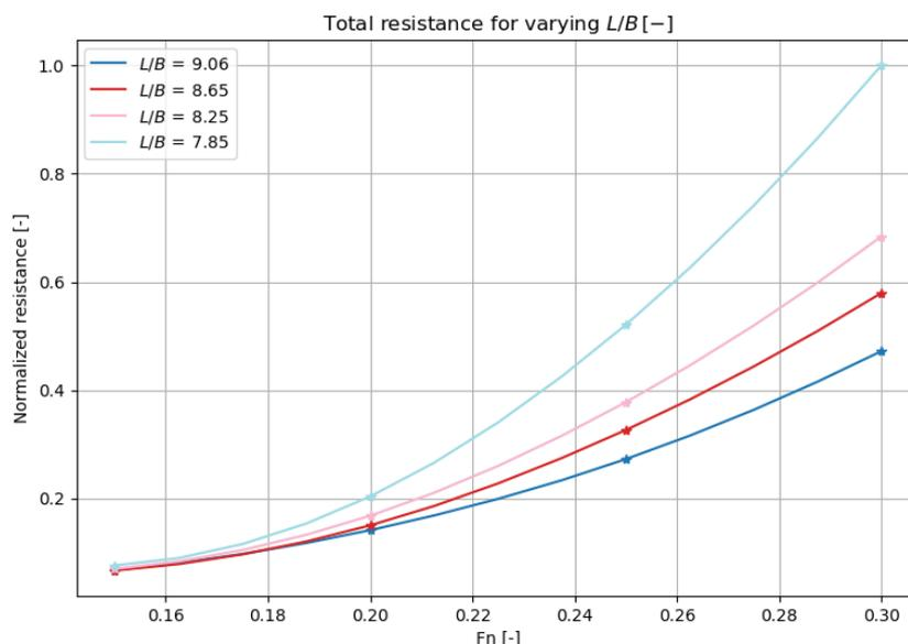
Figure 7-7: Total resistance results for hulls with various L/B-ratios created by varying the length.
