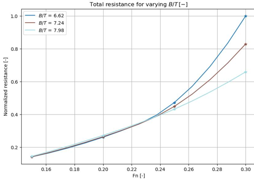
Figure 7-10: Resistance results for hulls with various  $B/T$ -ratios.
