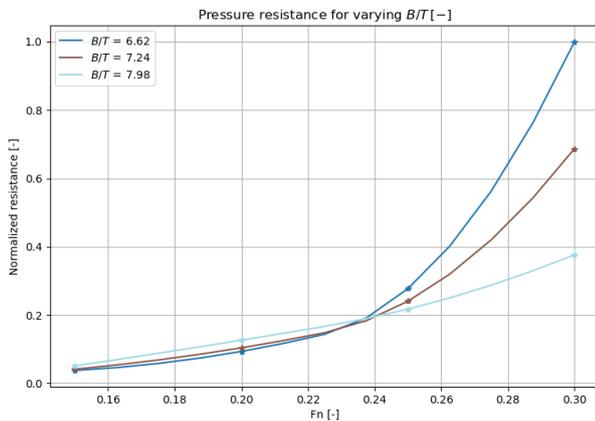
Figure 7-11: Pressure resistance for various  $B/T$ -ratios.
