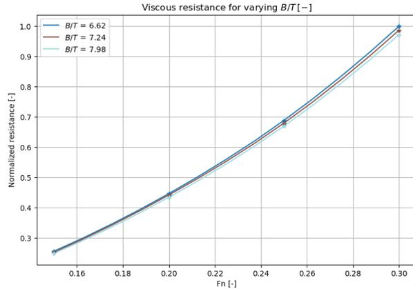
Figure 7-12: Viscous resistance for various  $B/T$ -ratios.
