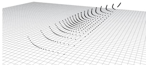
Figure 5-6: Example of evaluated surface points for a new hull shape.
