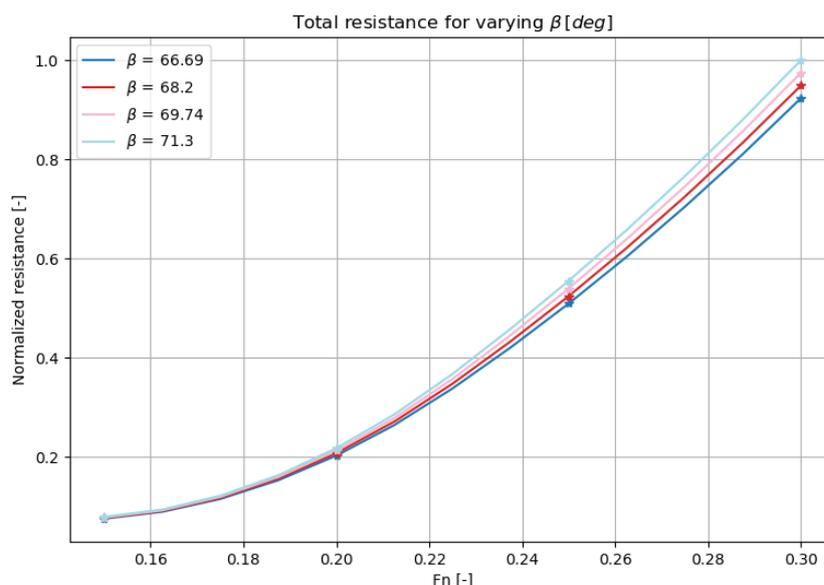
Figure 7-13: Resistance results for hulls with various entrance angles.
