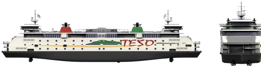
Figure 3-2: Design of the Dokter Wagemaker, a Damen-built double-ended road ferry [78].
