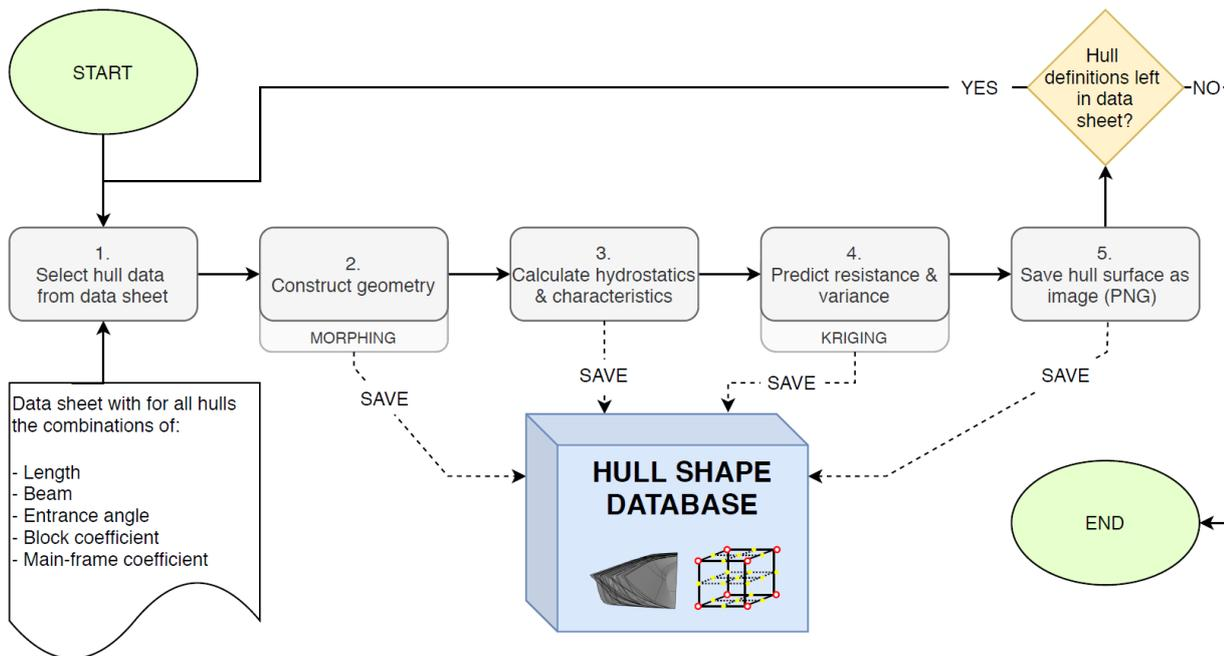
Figure 5-1: Approach to fill the database.
