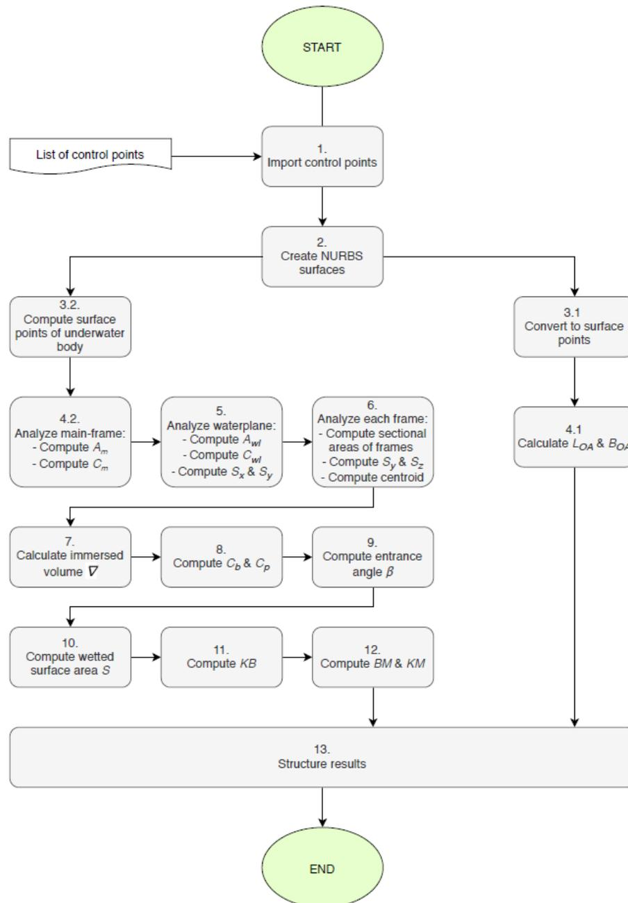
Figure 5-7: Procedure to calculate hydrostatics and other characteristics.
