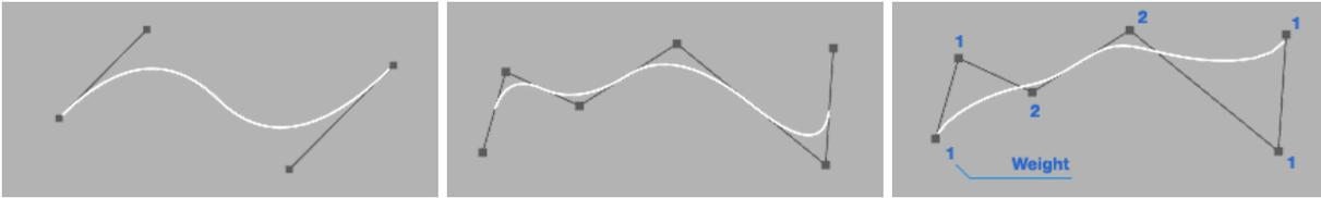
Figure 4-1: From left to right, a comparison between a Bézier spline, an open B-spline and NURBS with weighted control points [44].
