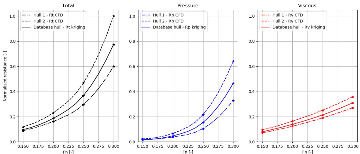
Figure 7-18: Resistance results for case 1.
