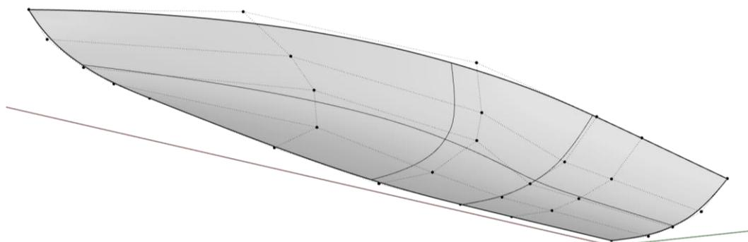
Figure 5-3: One quarter of the base hull with control points visible.
