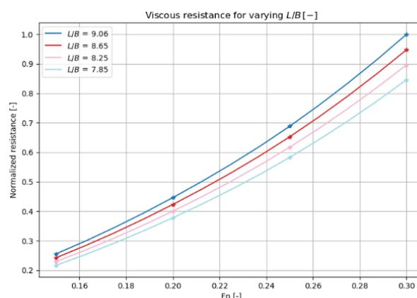
Figure 7-9: Viscous resistance for various L/B-ratios.
