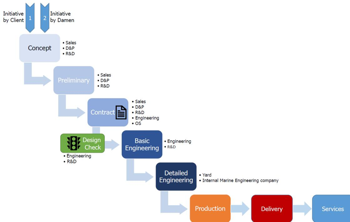
Figure 2-1: Phases in the ship design and production process within Damen including involved internal stakeholders.
