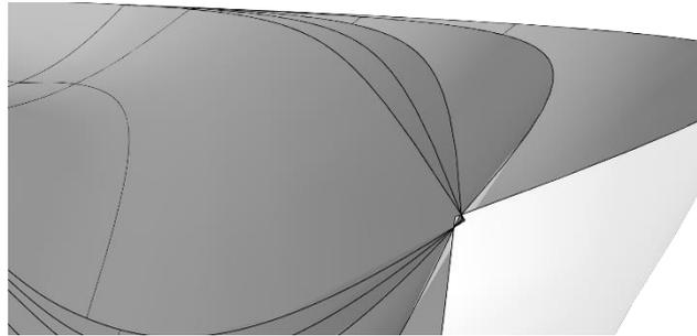
*Figure 7-6: Detailed view of the bow of hull shapes for varying entrance angle, showing that the length overall is also influenced by varying the entrance angle.*
