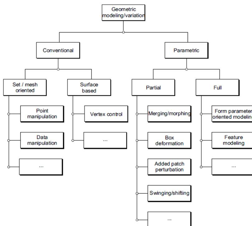
Figure 4-2: Possibilities for geometric modelling and variation [46].
