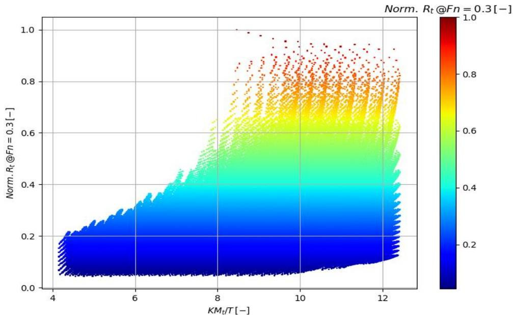
Figure 6-1: Maximum total resistance plotted versus the keel-metacentre distance divided by the draft.
