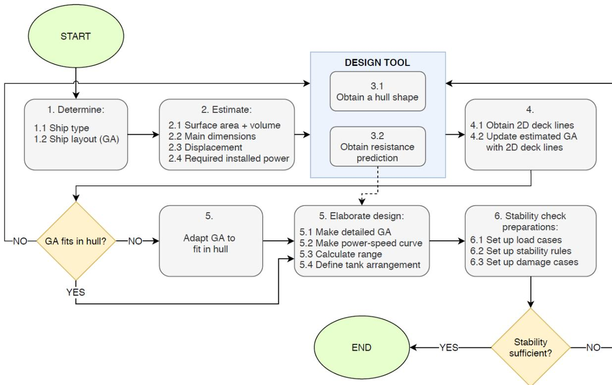
Figure 4-3: Placement of the design tool in the design process.
