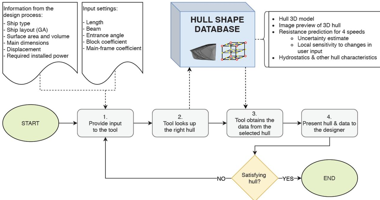
Figure 4-4: Overview of the tool working procedure.
