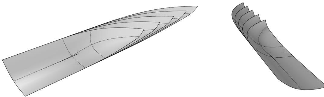
Figure 7-4: Geometries of hull shapes for varying length from two perspective views.
