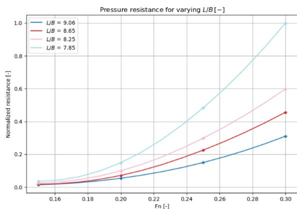
Figure 7-8: Pressure resistance for various L/B-ratios.
