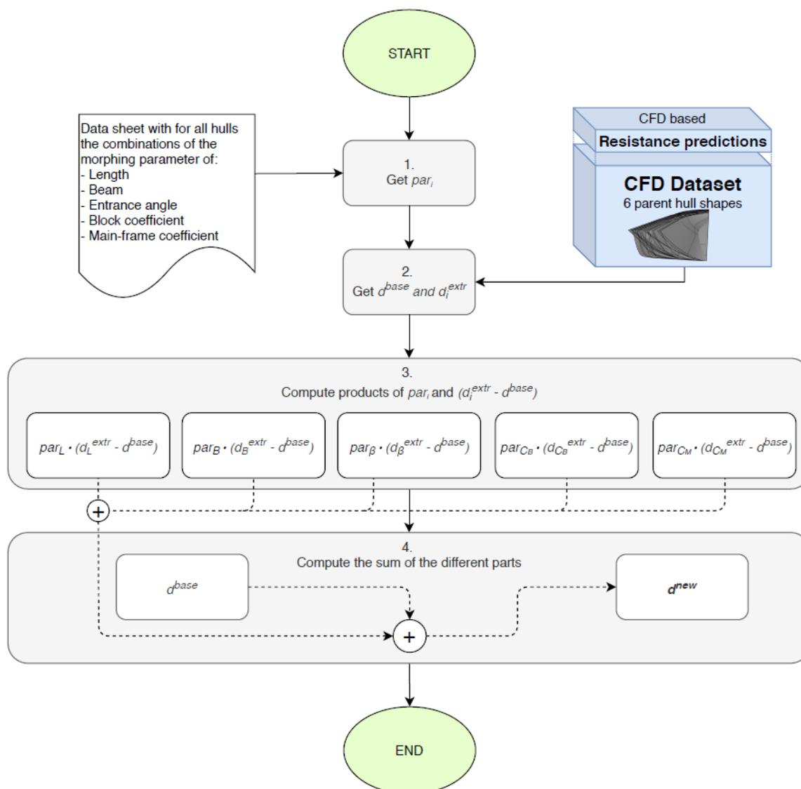
Figure 5-4: Procedure to obtain a new control point coordinate by morphing.
