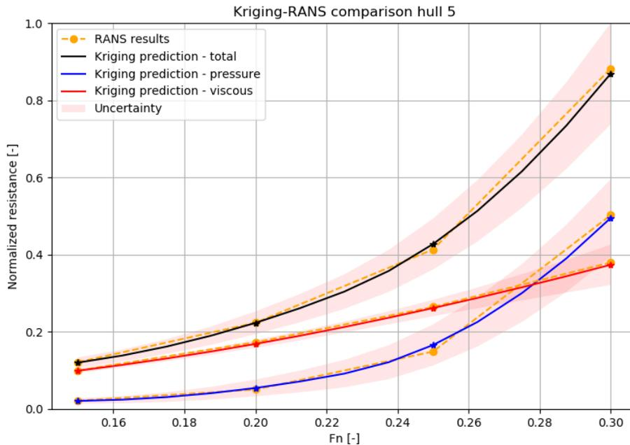
Figure 5-9: Normalized resistance components of the CFD results and kriging prediction for hull 5.
