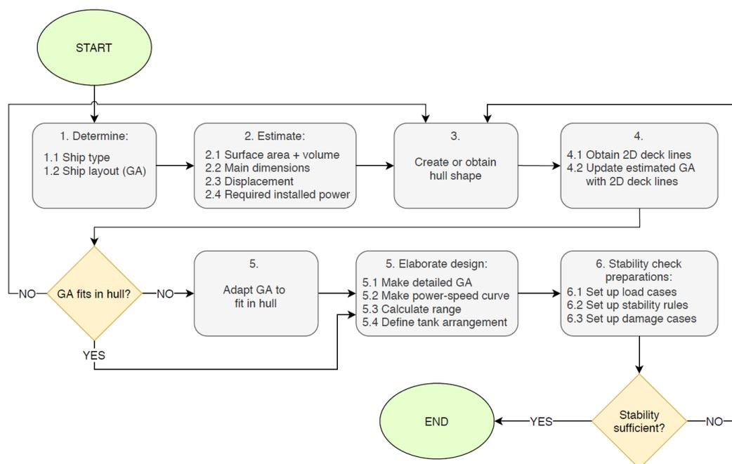
Figure 2-3: Concept design approach for OPVs within Damen.
