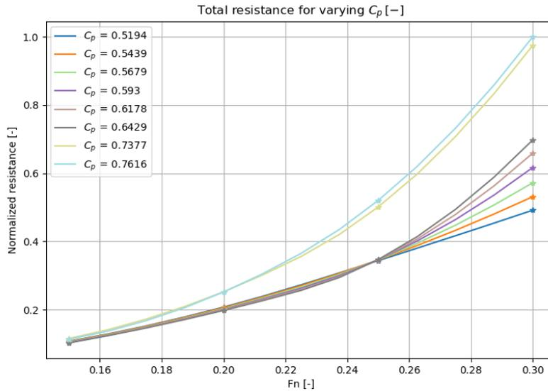
Figure 7-15: Resistance results for hulls with various prismatic coefficients.
