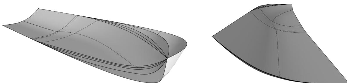
Figure 7-5: Geometries of hull shapes for varying entrance angle. The right picture shows that the main-frame coefficient is also influenced by varying the entrance angle.
