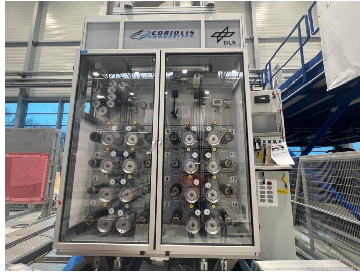
Figure 4.5: Creel system of the Coriolis C1 ADFP unit
