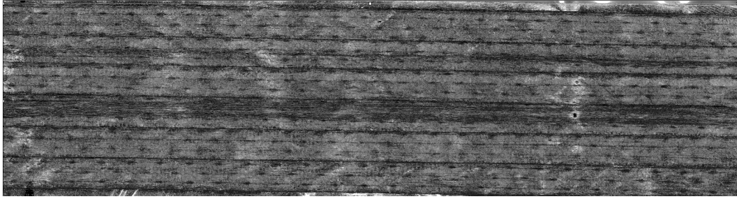
Figure 5.19: Microscope image of a slightly frayed specimen of group 4
