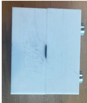
Figure 5.16: 3D printed clamp for cross-sectional dry fibre specimen
