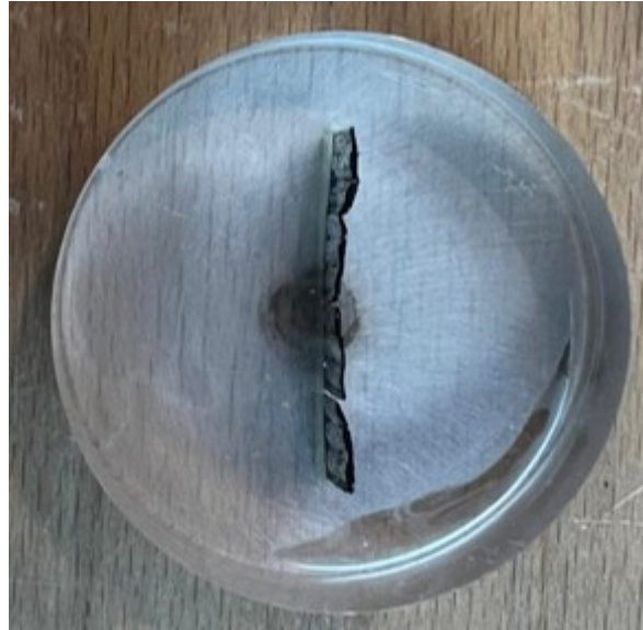
Figure 5.14: resin cast specimen for cross-section microscopy
