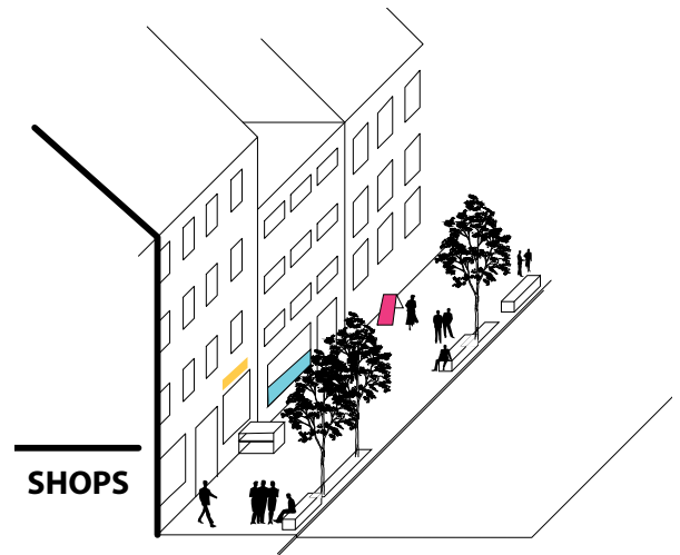
Figure 130. Section of proposed potential attractor street showing trees and benches as recognizable elements and shop owner personalization
