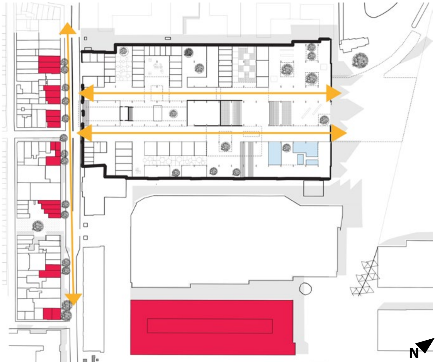
Figure 125. Map of proposed design with major pedestrian connections to increase the flux of people
